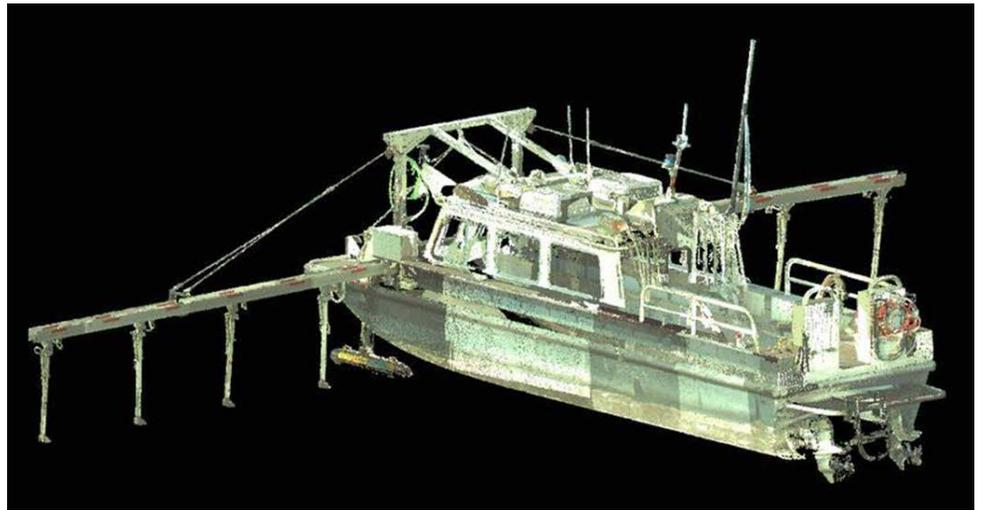
**This scan of the Motor Vessel Hines allowed the District to obtain offset calculations between the new GPS receivers and the bow-mounted sounding equipment.**
