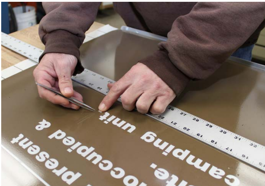
Maintenance mechanic, Shay Bevens, uses tweezers to place a small piece of vinyl lettering on a sign being produced at the Sign Shop.
