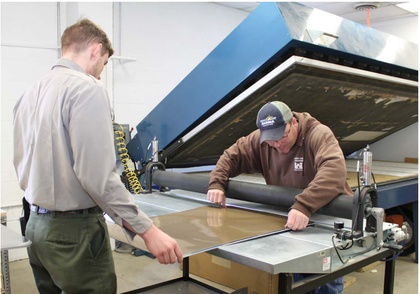
Justin Lind (left) and Shay Bevens (right) carefully place a sheet of vinyl backing material on an aluminum blank to begin the sign making process at the District's Sign Shop at Coralville Lake. Photo by Samantha Heilig
