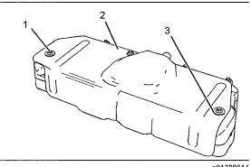
If the valve mechanism cover is equipped with a heat shield, remove bolts (1) and washers (3) from heat shield (2).
