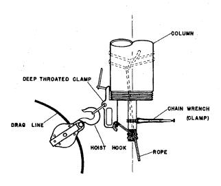
Figure 5-2 Product Lubrication Column Hoisting
