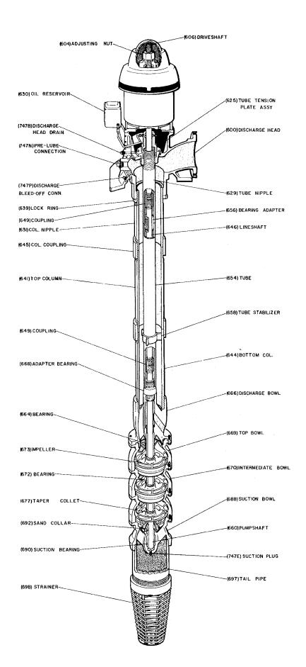
Figure 6-1 Enclosed Lineshaft Pump
