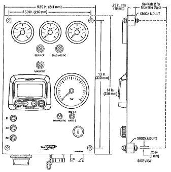
NOTE 1: Flat Panel has approximately 8 inch leads on connectors. Typical application shown, features vary per engine application.
