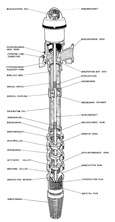
Figure 5-1 Product Lubrication Pump
