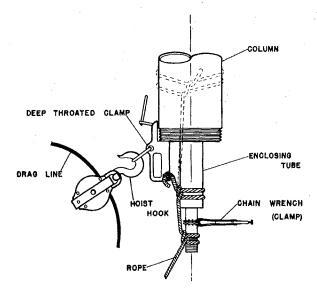
Figure 6-2 Oil Jubrication Column Hoisting
