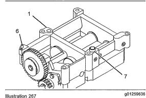
8. Do not remove dowel (6) and dowel (7) unless the dowels are damaged.
