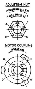
Figure 10-2 Impeller Adjustment
