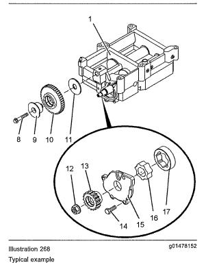
2. Remove bolt (8) and hub (9). Remove idler gear (10) and thrust washer (11).
