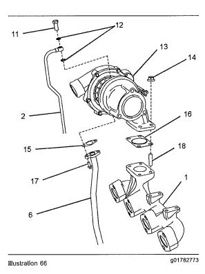
Clean the gasket surfaces of the exhaust manifold (1). If necessary, install studs (18) to the exhaust manifold. Tighten the studs to a torque of 18 N·m (13 lb ft).
