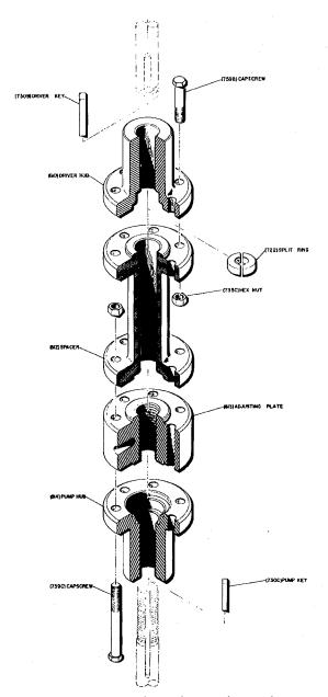
Figure 11-2 Flanged Adjustable Coupling with Spacer
