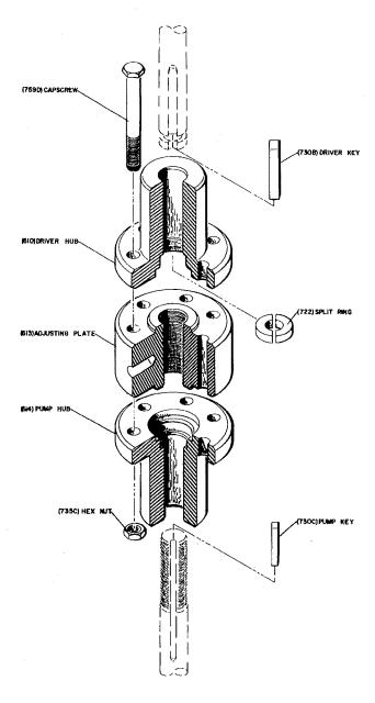
Figure 11-1 Flanged Adjustable Coupling
