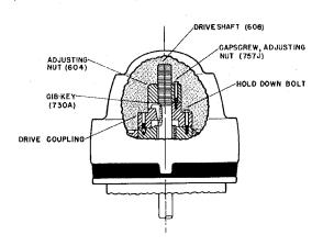
Figure 10-1 Hollow Shaft Adjusting Nut
