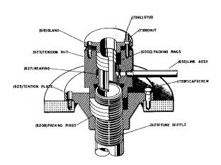
Figure 9-2 Tension Plate Assy (Flush Lubrication)
