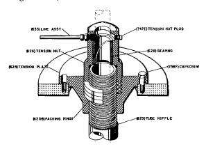
Figure 9-1 Tension Plate Assy (Drip Feed Lubrication)
