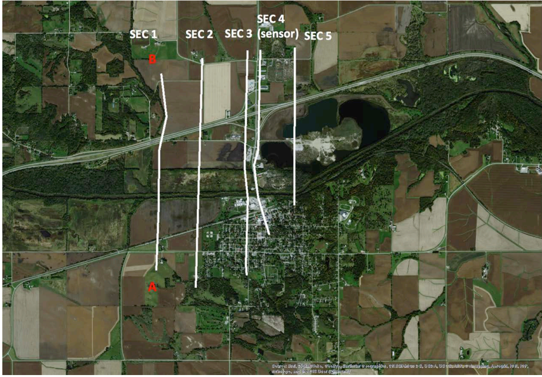
Figure 5b. Cross-sections surveyed next to the South Skunk River bridge at Colfax.
