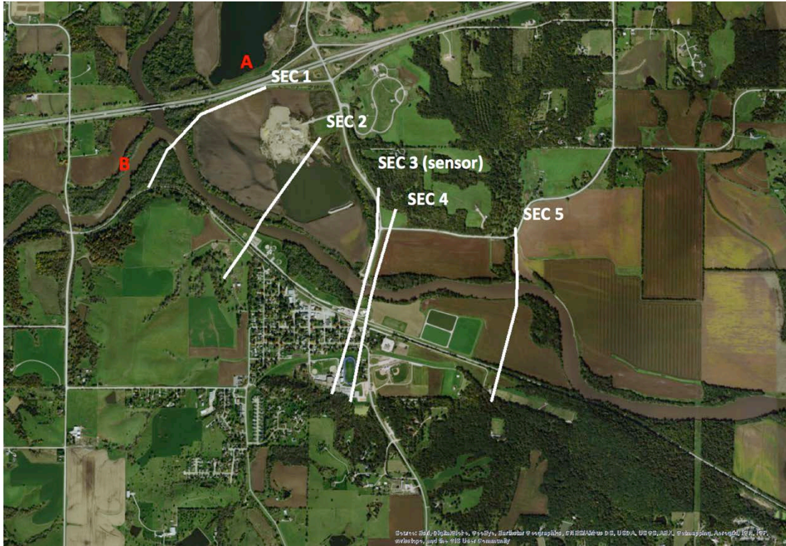
Figure 5c. Cross-sections surveyed next to the Raccoon River bridge at Van Meter.
