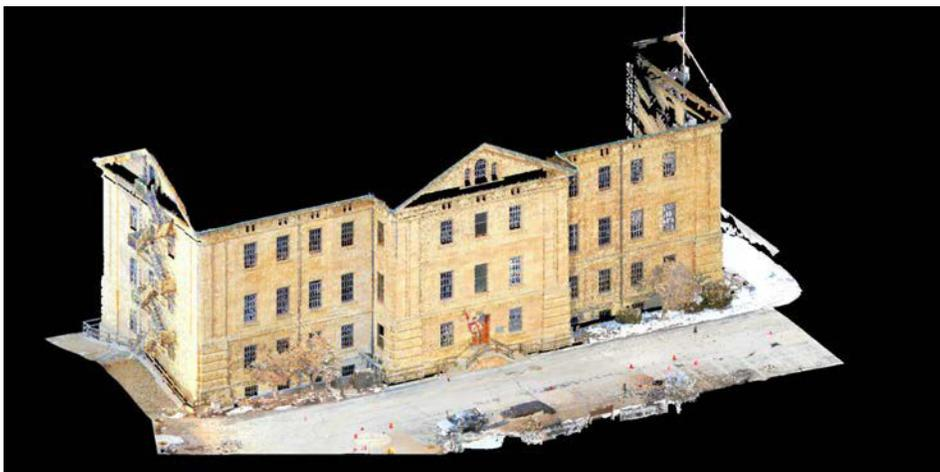
**The initial high density scan of the front of the Clock Tower Building viewed with Leica Cyclone software.**
