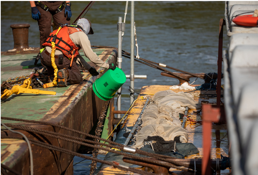
A representative from the U.S. Fish and Wildlife Service manually dumps a calculated number of fish between two barges during automated barge clearing deterrent testing at Peoria Lock and Dam. This action was done to measure the effectiveness of the system.
