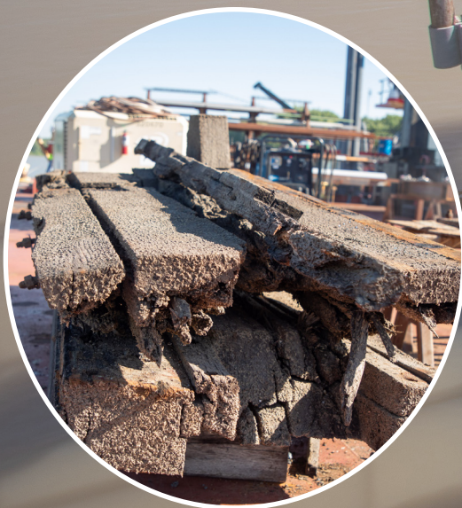
Remnants of used wicket gates after being pulled from the Illinois Waterway. Photo by Kelcy Hanson
