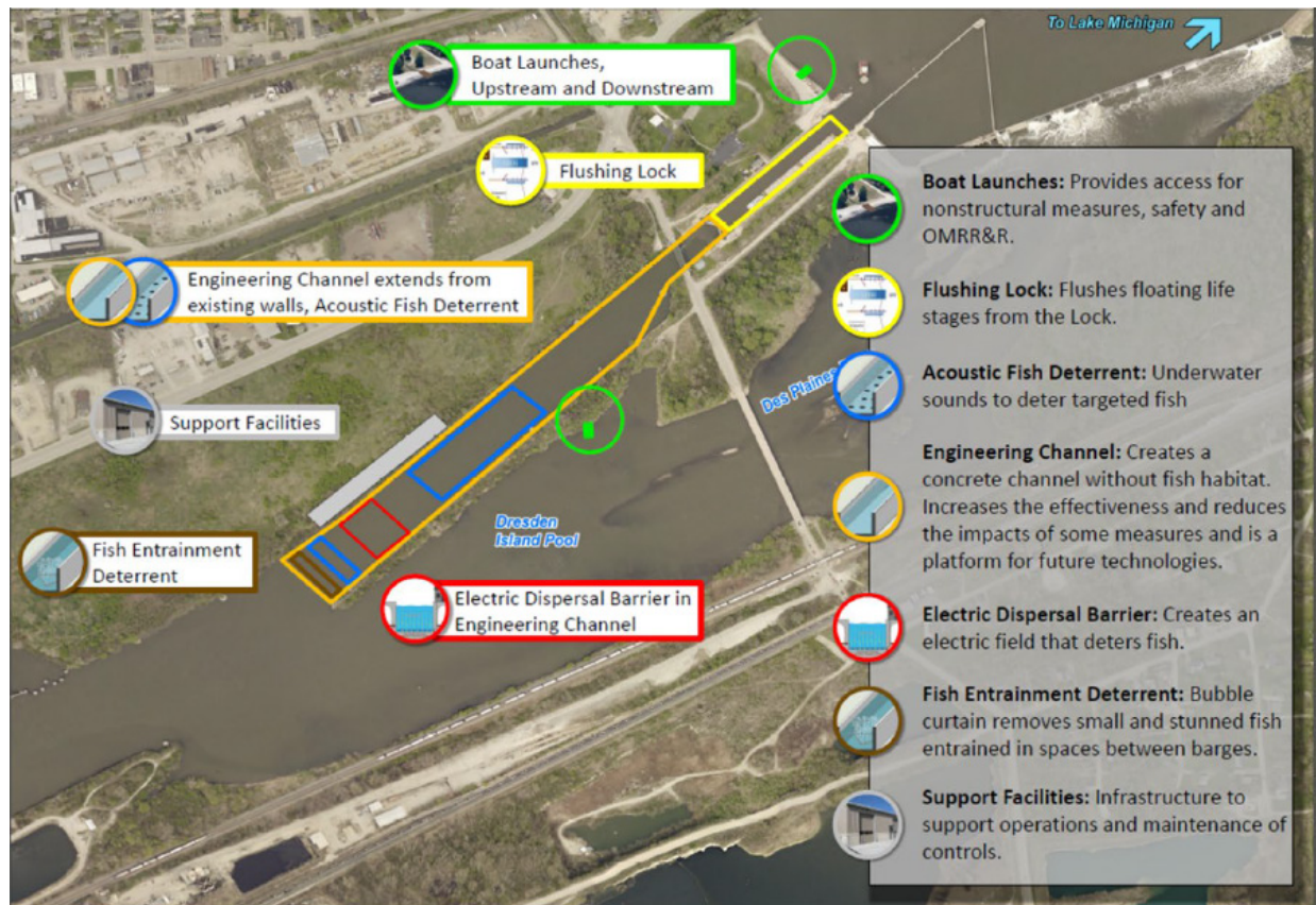
Figure 2.2. All Brandon Road Project Features
