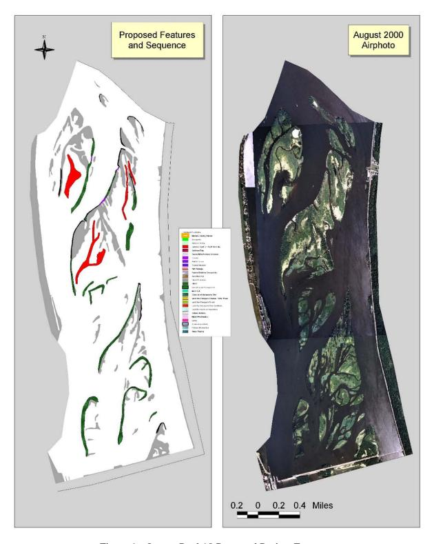
Figure 1 – Lower Pool 10 Proposed Project Features
