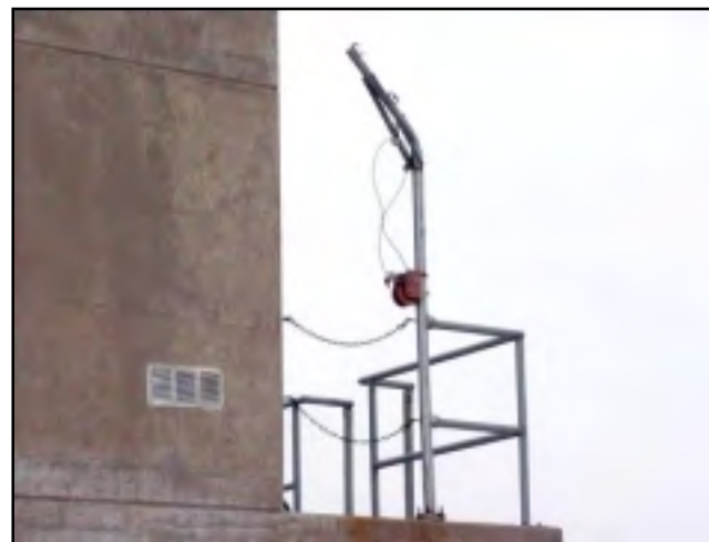
Manual hoist & jib crane mounted to handrail
