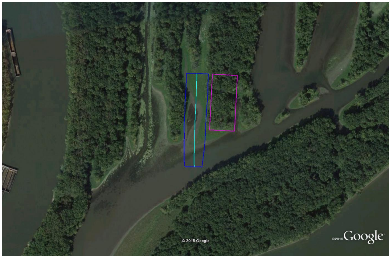
Figure 3. “Small lake” Dredge Cut Proposed Alignment and Material Placement
