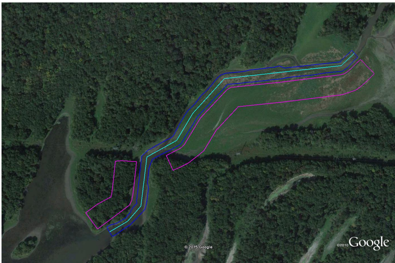
Figure 7. Upper Lake Dredge Cut Proposed Alignment and Material Placement
