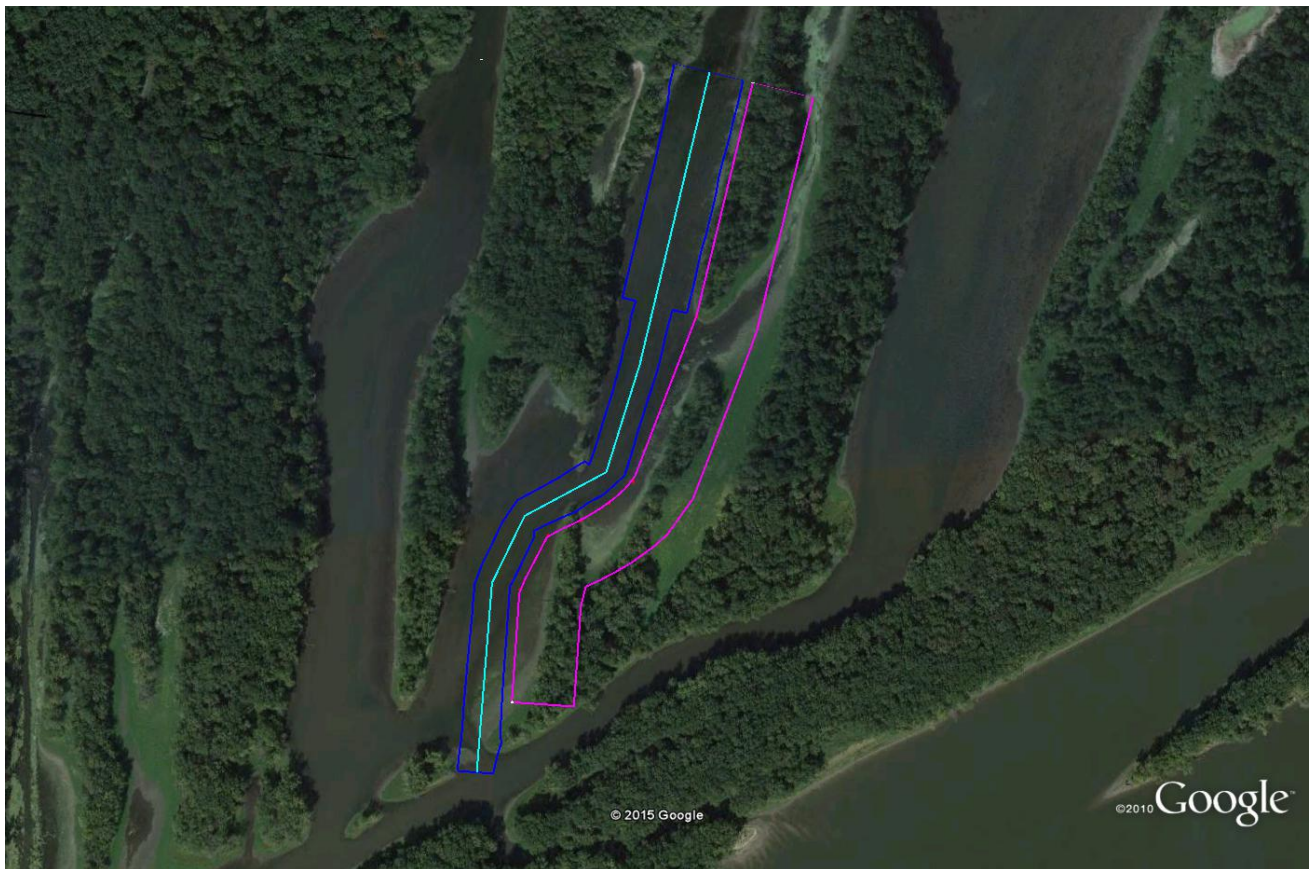
Figure 5. Sand Burr Dredge Cut Proposed Alignment and Material Placement
