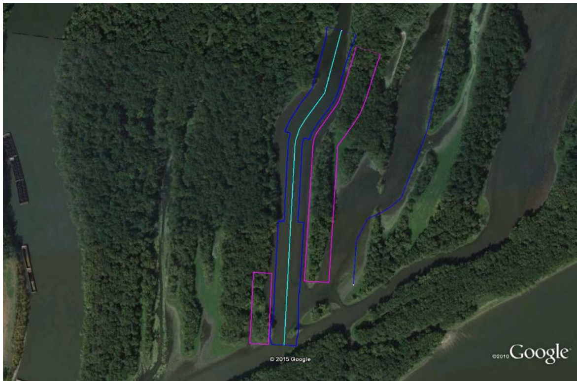
Figure 4. Blue Bell Dredge Cut Proposed Alignment and Material Placement
