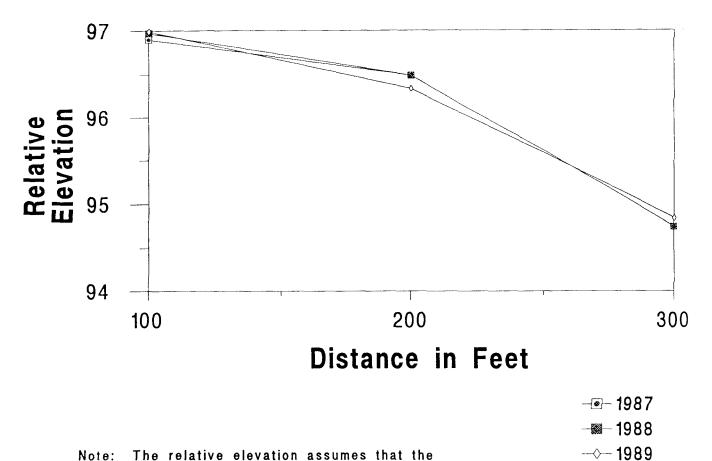
Note: The relative elevation assumes that the bench mark which the soundings are referenced to is at an elevation of 100.
