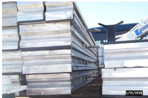
35. Lake Chautauqua. 6 inch and 12 inch aluminum stop logs. 10 ft long.
