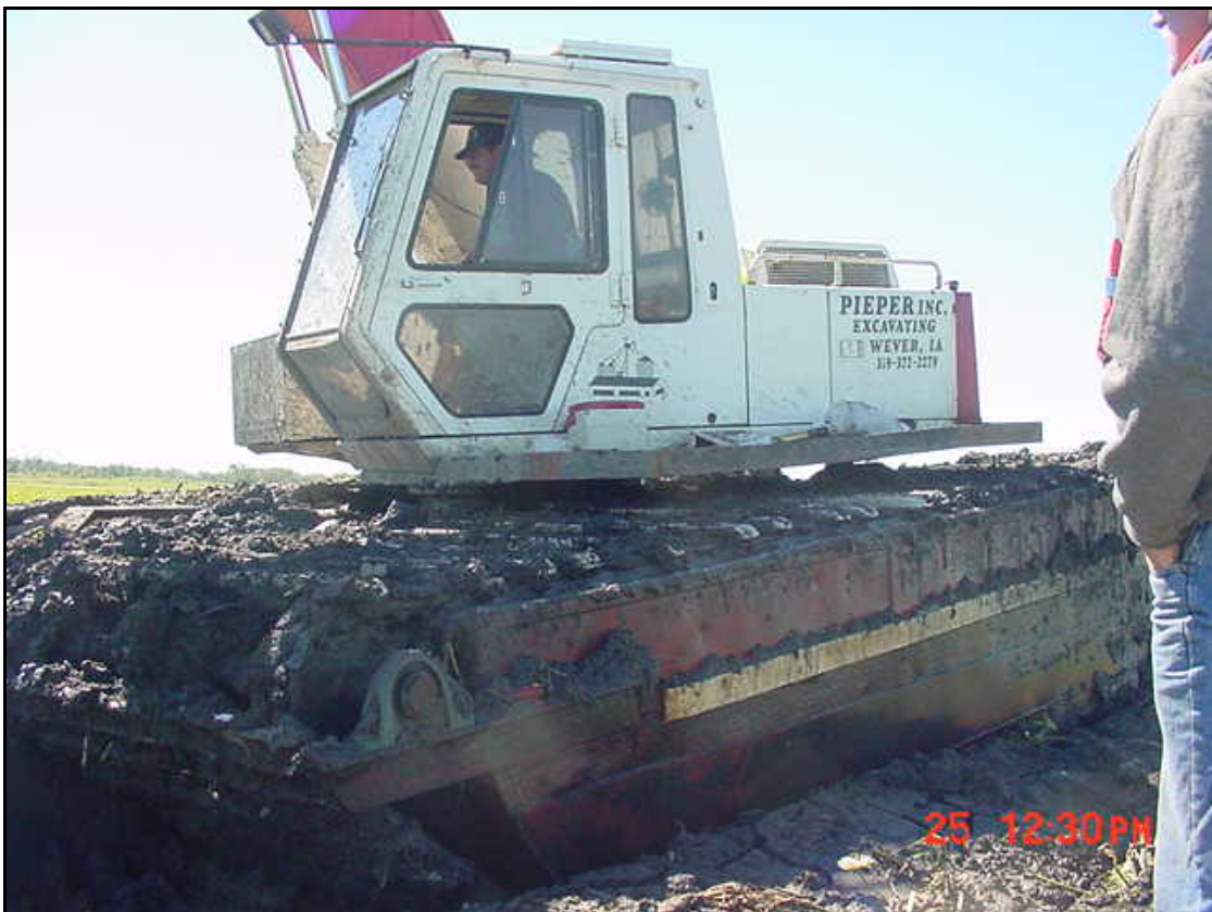
Photograph C-14. Floating Excavator used for Lower Lake Channel
