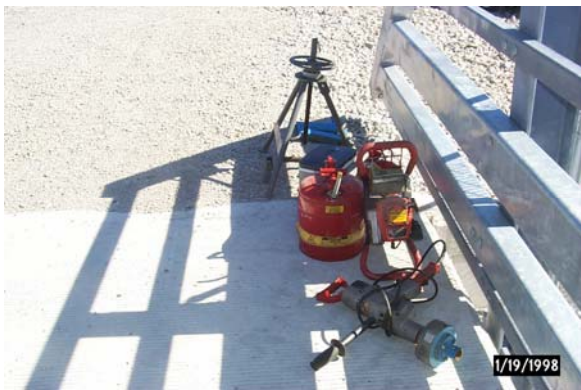
32. Lake Chautauqua. Gas and Electric portable operators for both pump station gates and water control structure gates.
