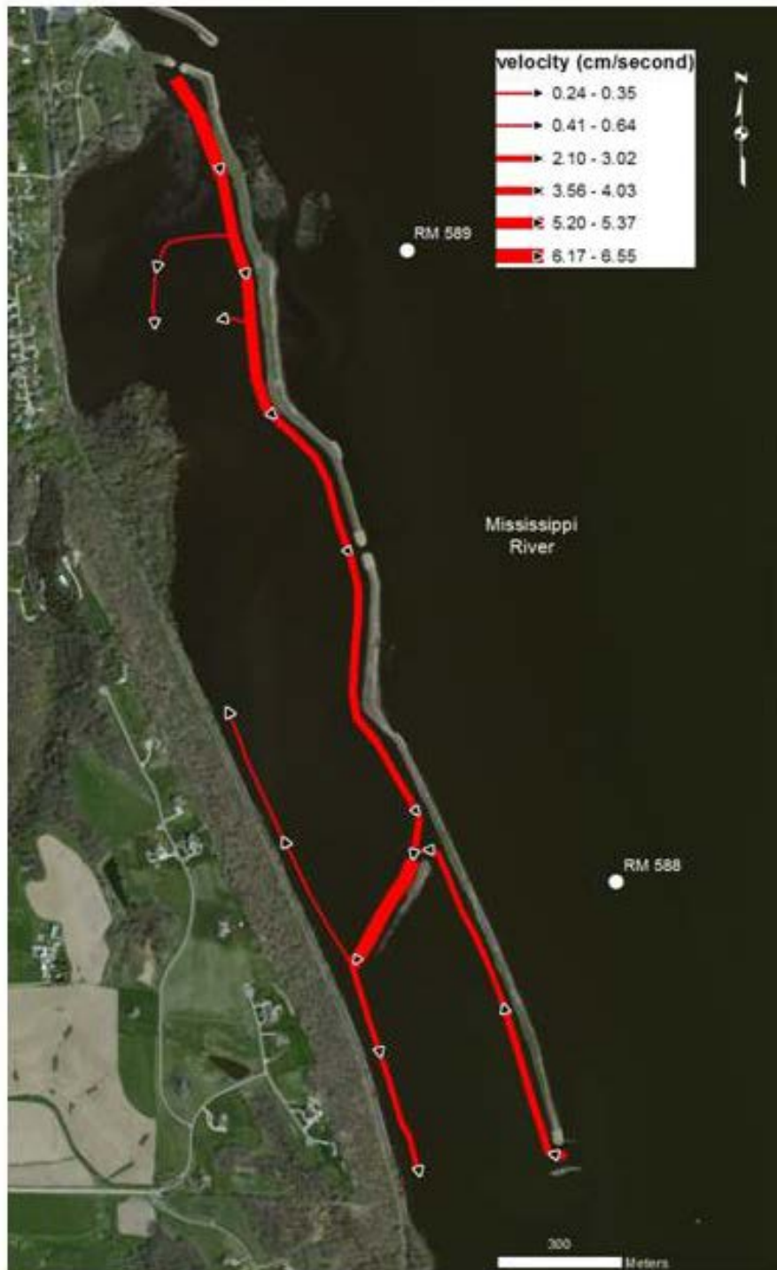
Figure 6. Recalibrated RMA2 hydraulic model following a 2014 dye study at Mud Lake HREP, Dubuque County, Iowa. Line thickness indicates relative velocity.
