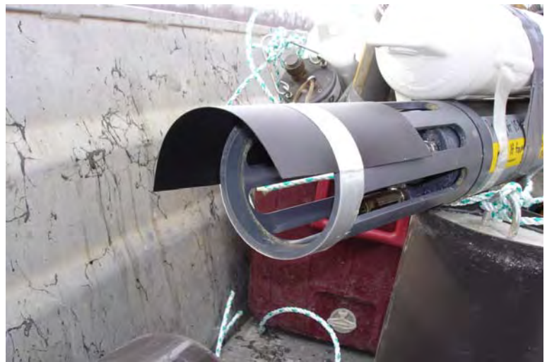
Figure 5. Sonde fitted with plastic shade to reduce exposure to sunlight.
