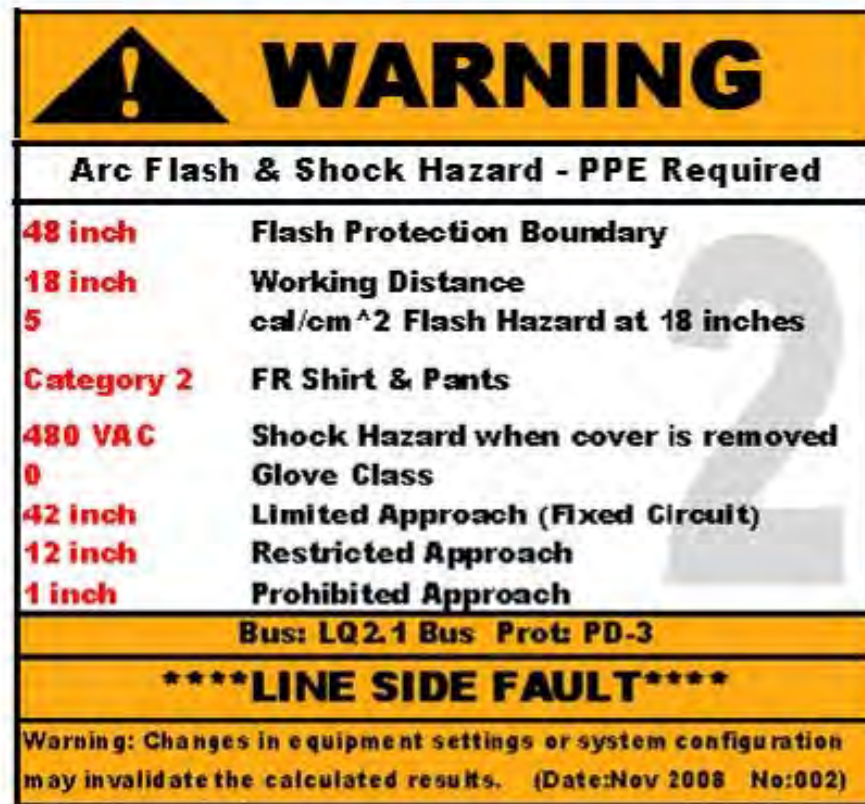
Arc Flash Hazard (AFH) Warning Label – USACE Format Required by ER and EP 385-1-100
