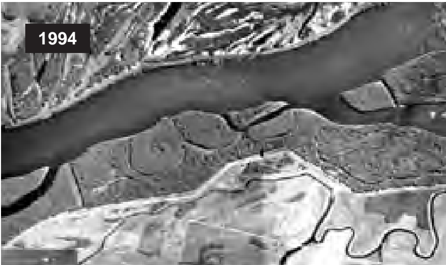
Filling between wing dams decreases main channel area.
