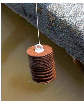
Figure 4. Hester-Dendy sampler (image:
