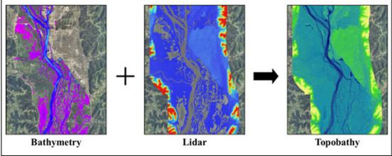
Bathymetry + Lidar = Topobathymetry
