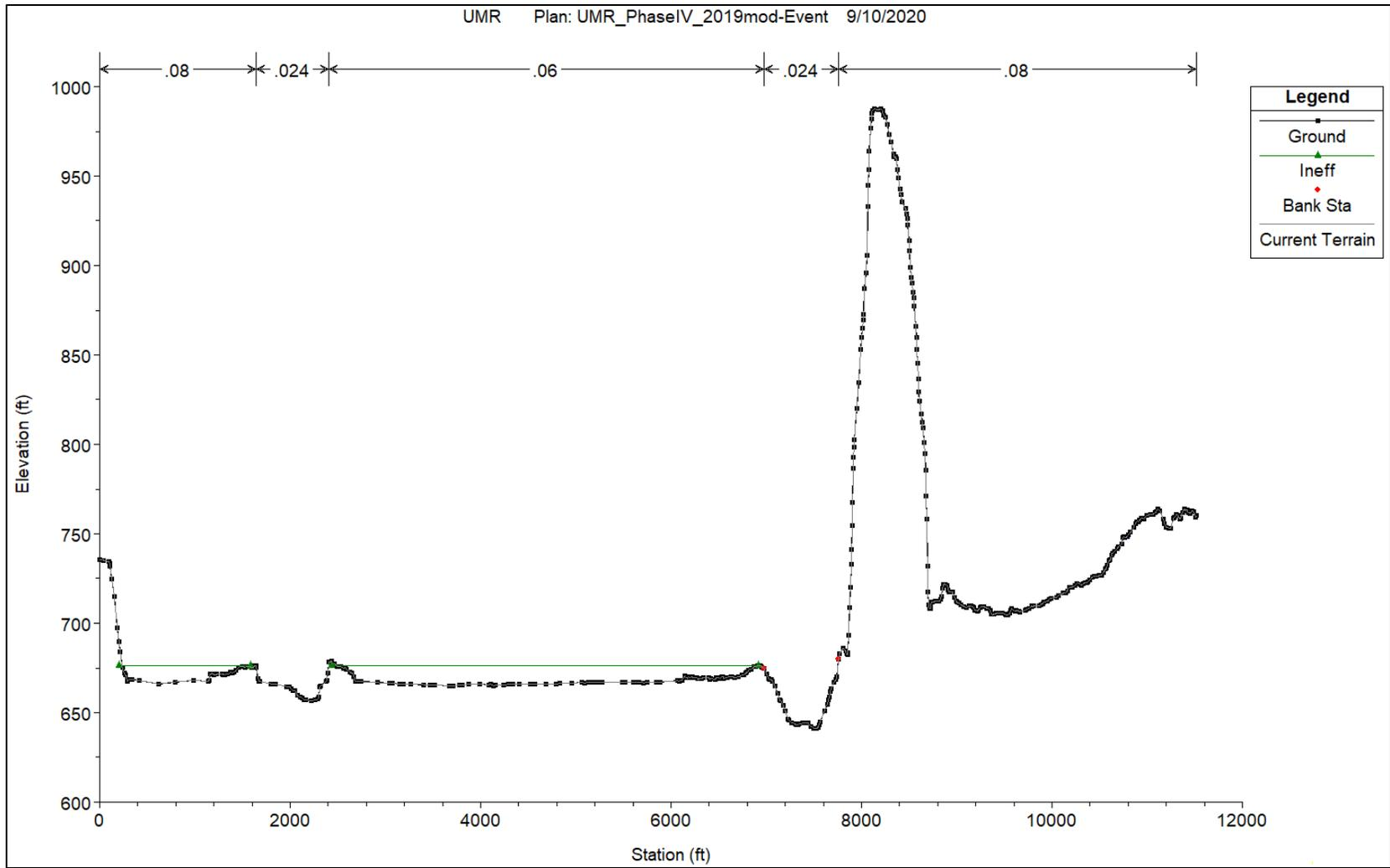
**Figure 2. Example Cross Section from HEC-RAS with Manning Roughness Coefficients Displayed Along Top of Cross Section**
