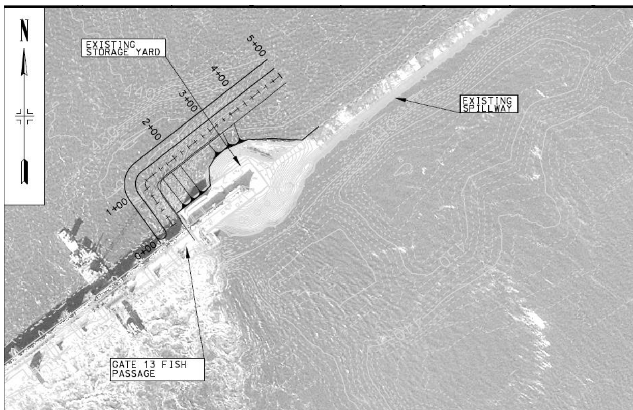
Figure 12. Measure E8: Rock Ramp Through Gate 13, Upstream of the Dam
