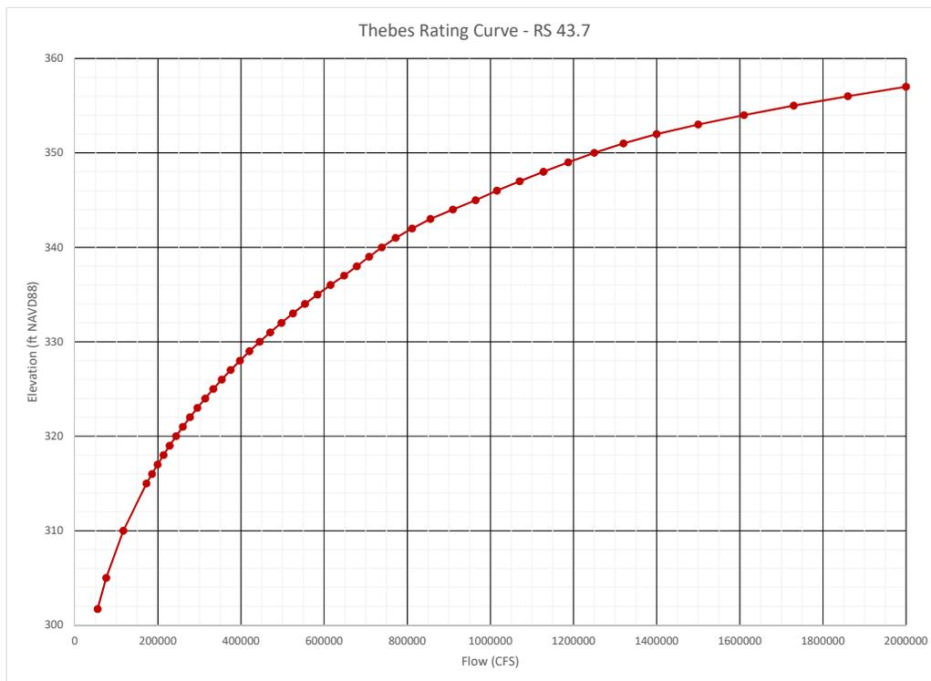
Figure 11 Rating curve used for the downstream boundary condition at Thebes, IL for the model application runs.
