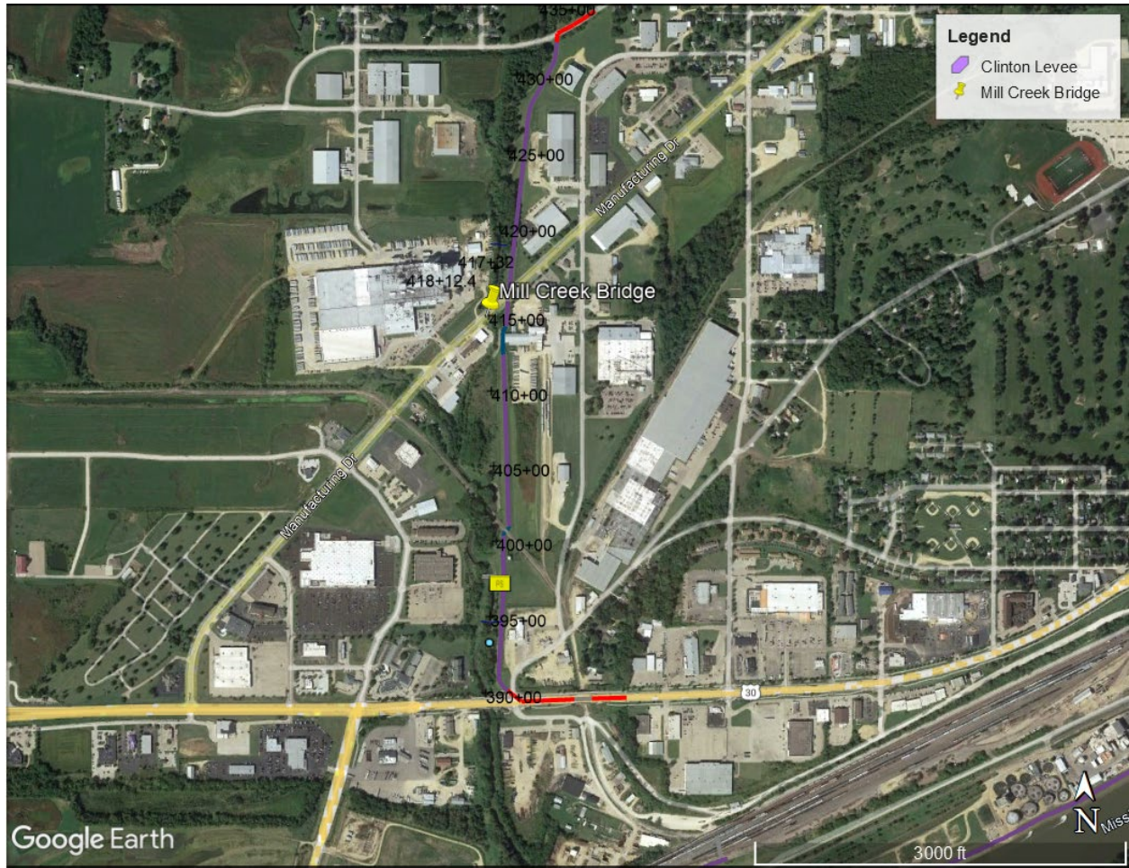
Figure 2. Project site map depicting the Mill Creek Bridge on Manufacturing Drive crossing the Clinton Local Flood Protection Project in Clinton, IA.
