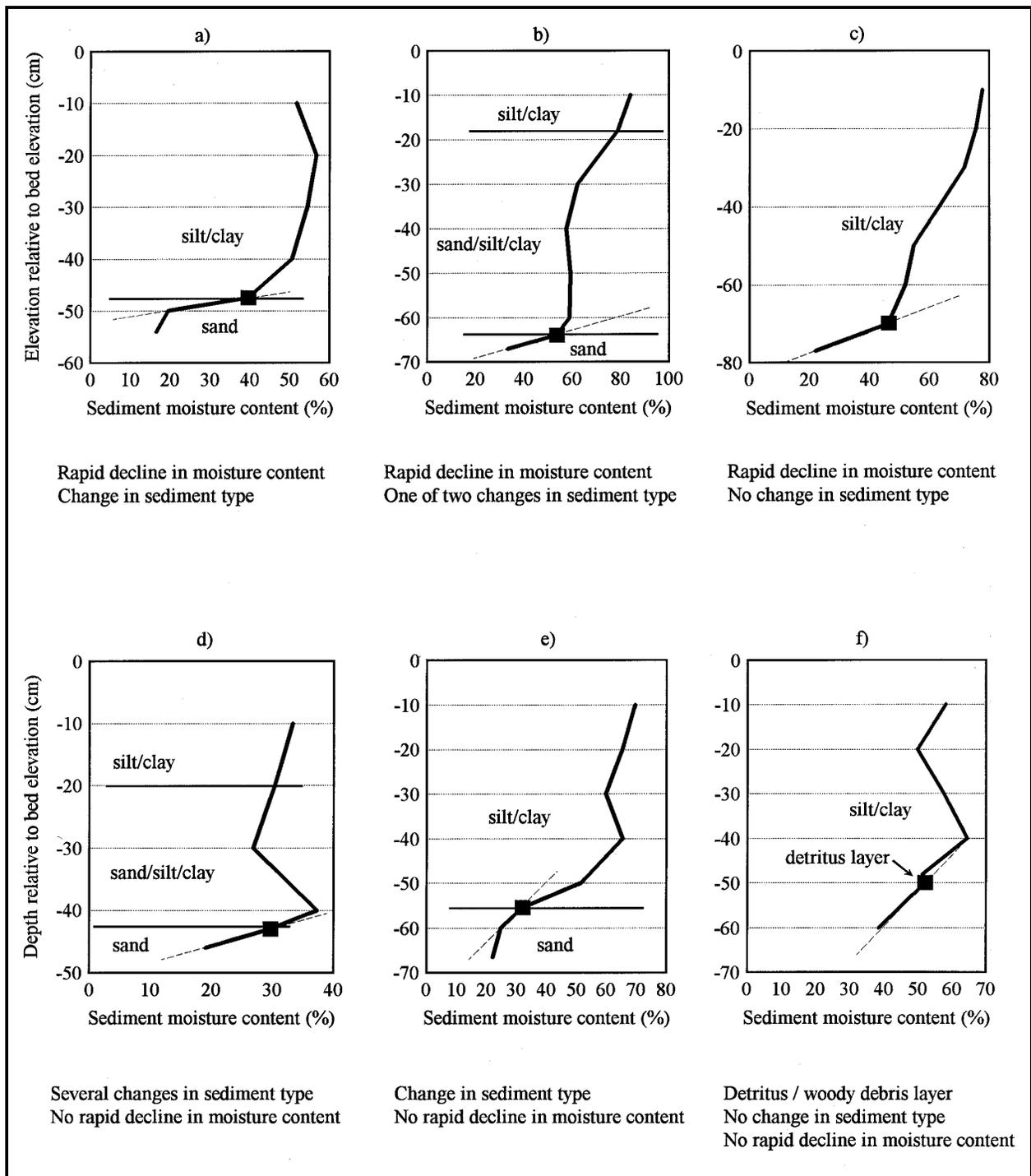
Figure 3. Examples of criteria used to identify preimpoundment sediment in the sediment cores. (Decline in moisture content is depicted by slope of dashed line in each graph; more horizontal lines indicate a rapid decline in moisture content. Sediment types are labeled above and below the switch as marked with the solid horizontal lines)
