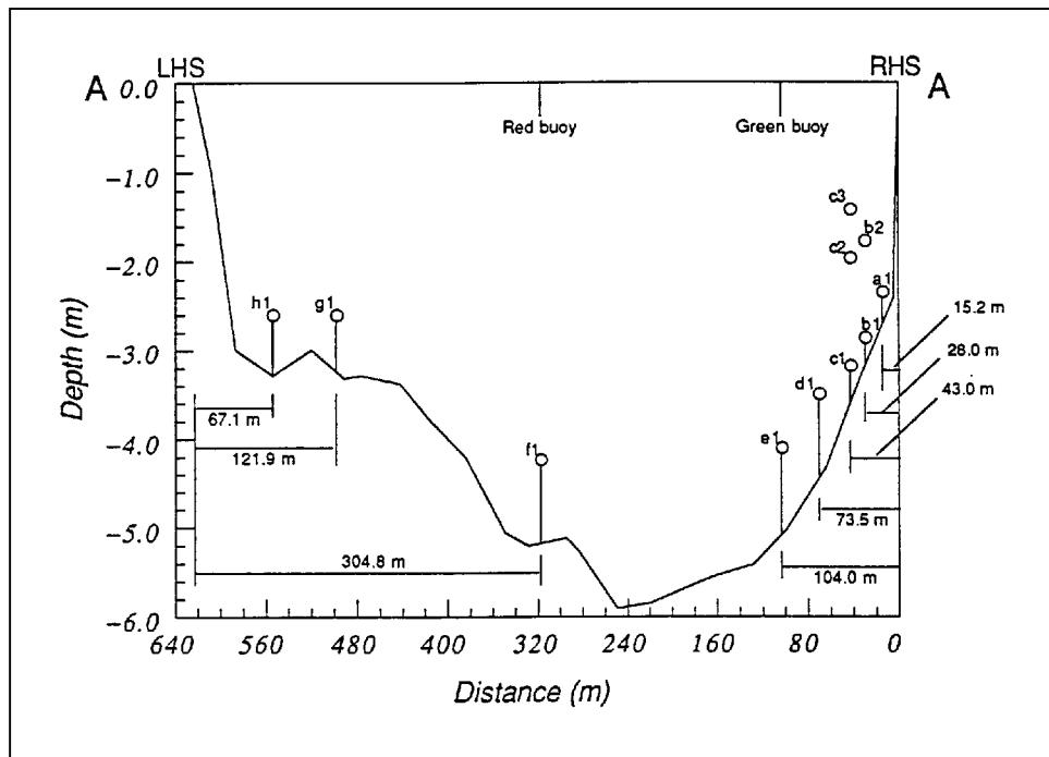
Figure 2. Cross section of the Mississippi River at the Clark's Ferry site for trip 1
