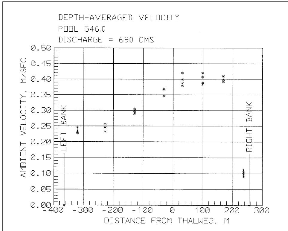
Figure 13. Depth-averaged ambient velocity distribution for Pool 546.0,  $Q = 690 \text{ cms}$
