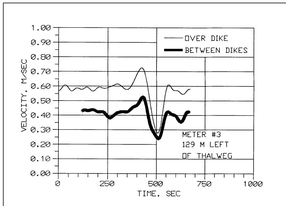
Figure 95. Velocity time history, downbound tow, meter No. 3, tow speed relative to ground = 4.77 m/sec
