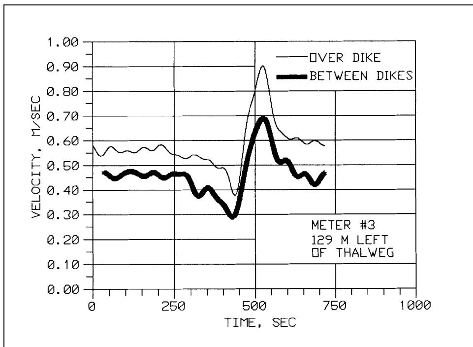
Figure 93. Velocity time history, upbound tow, meter No. 3, tow speed relative to ground = 4.16 m/sec
