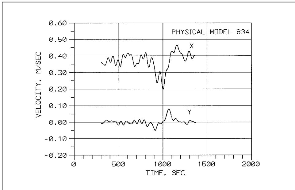
Figure 21. Velocity time history for *Coop Ambassador*, Probe number 834, physical model data
