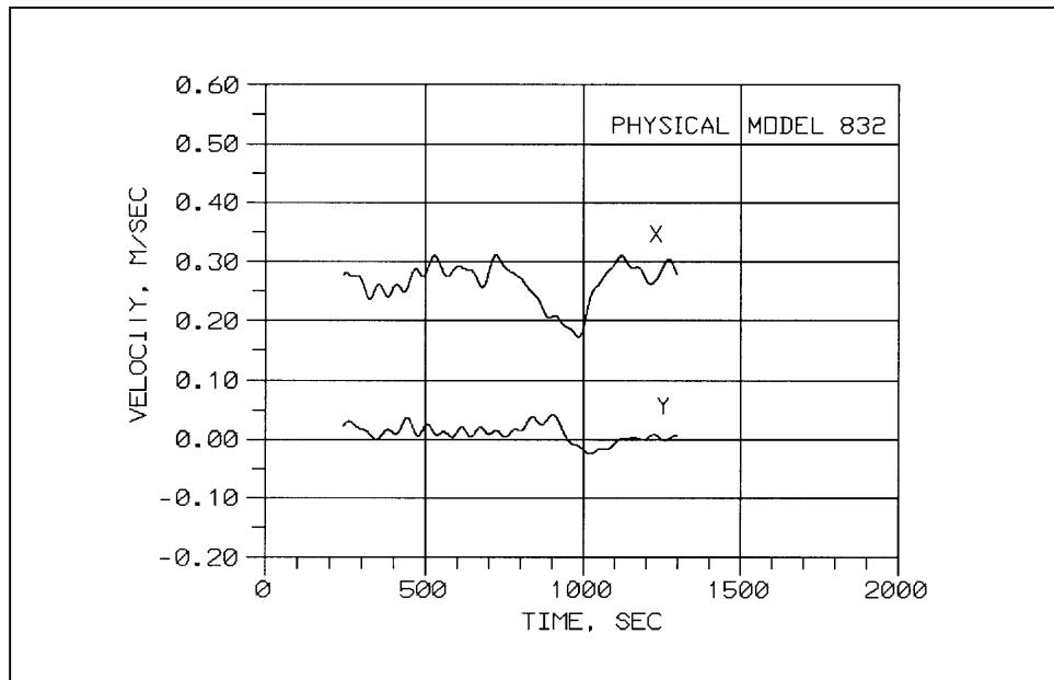
Figure 17. Velocity time history for *Coop Ambassador*, Probe number 832, physical model data
