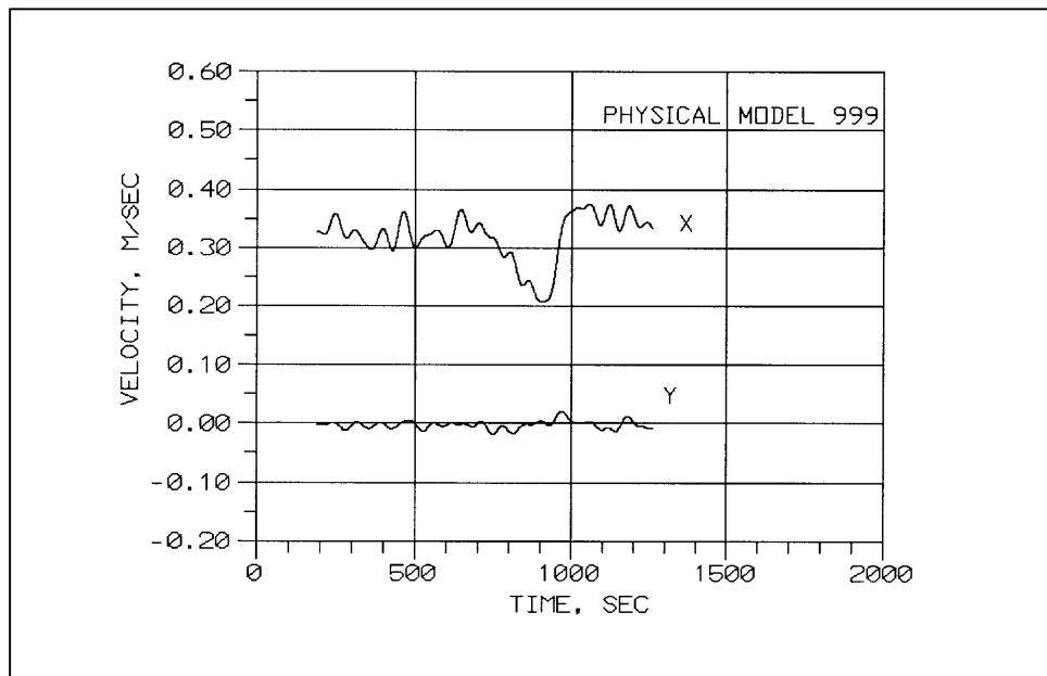
Figure 25. Velocity time history for *Coop Ambassador*, Probe number 999, physical model data
