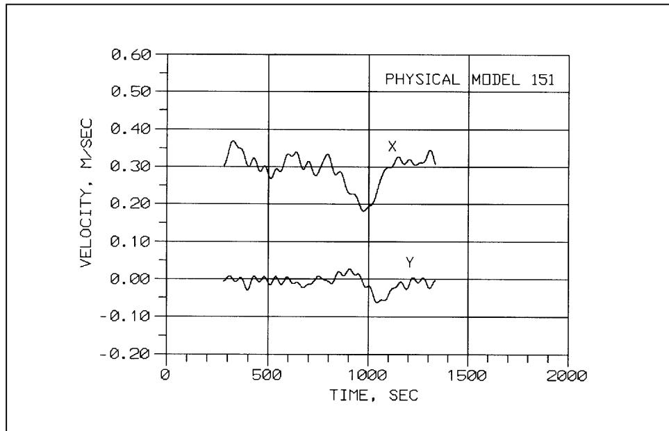
Figure 19. Velocity time history for *Coop Ambassador*, Probe number 151, physical model data
