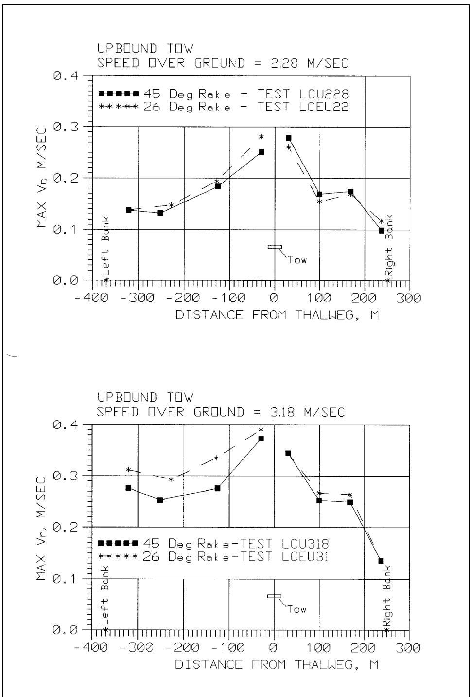
Figure 76. Return velocity, rake angle effects, upbound tow
