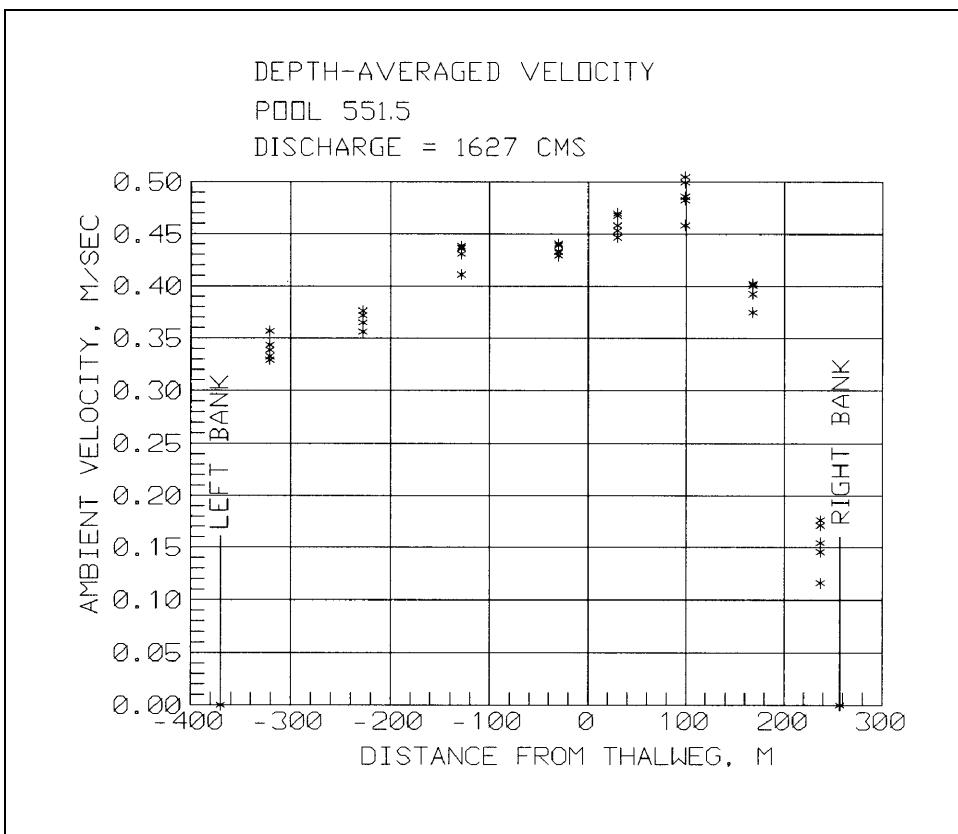
Figure 78. Ambient velocity distribution, experimental series 5
