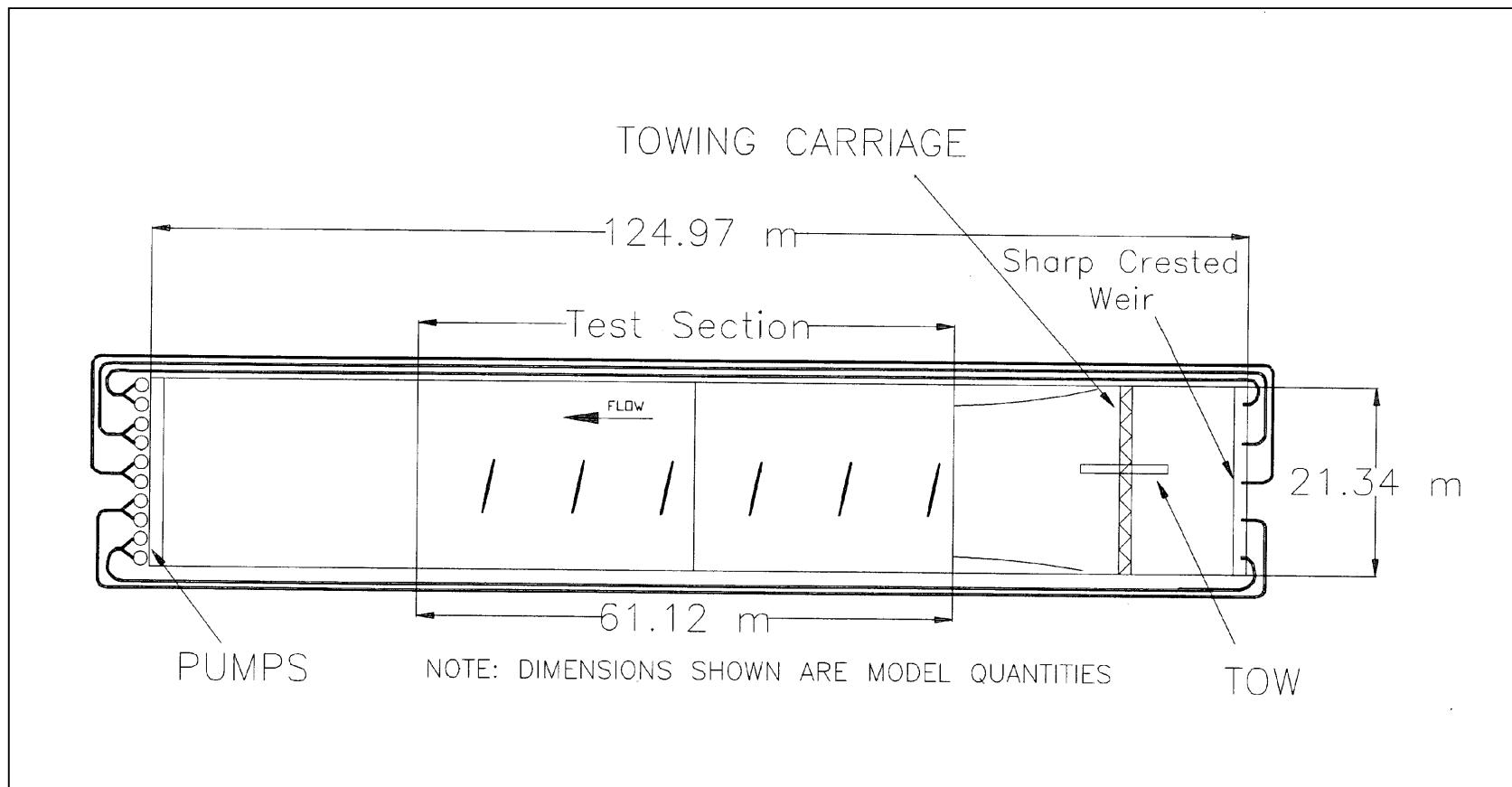
Figure 7. Schematic of navigation effects model
