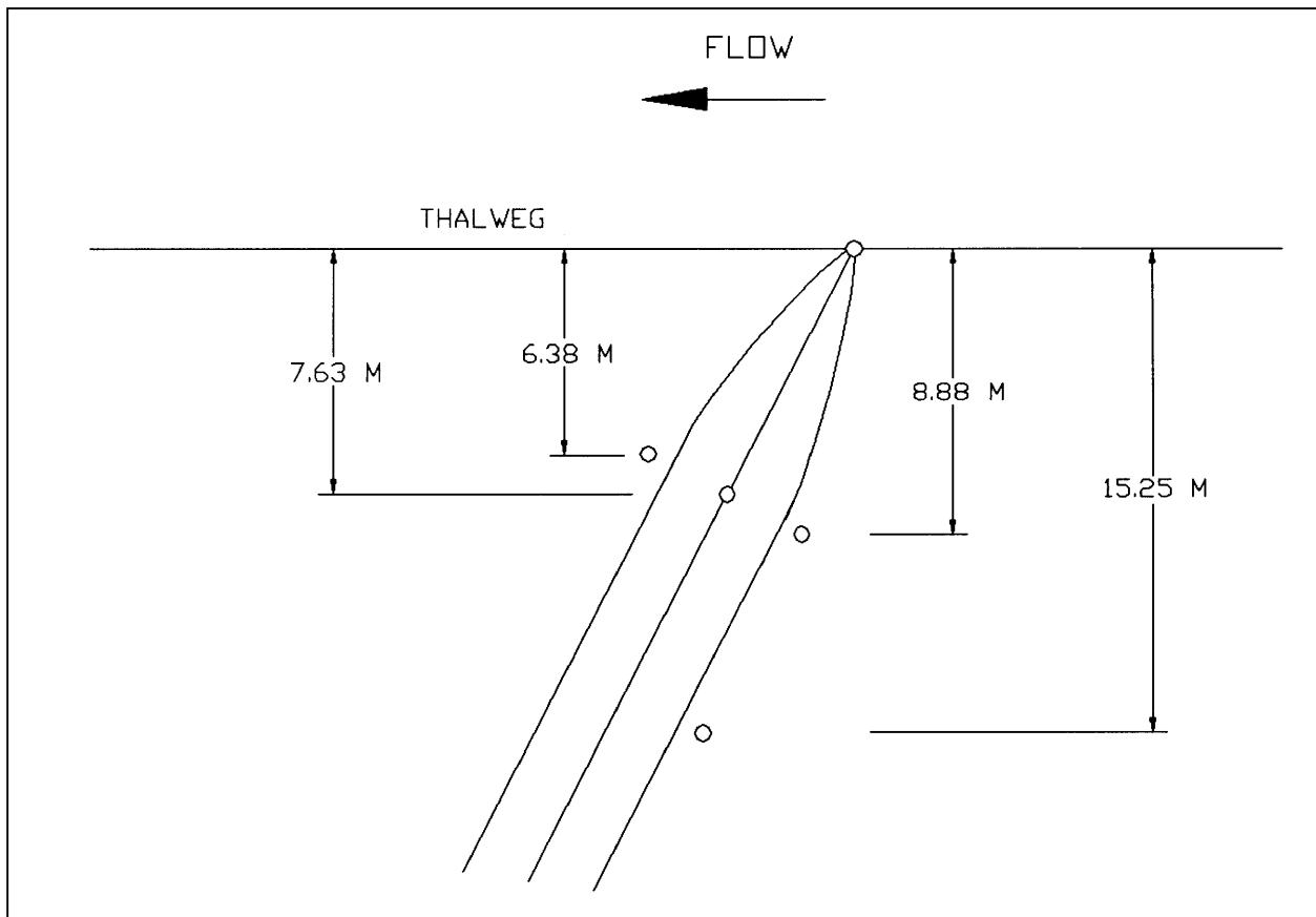
Figure 97. Location of velocity meters in dike experiments
