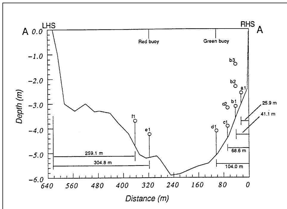
Figure 3. Cross section of the Mississippi River at the Clark's Ferry site for trip 2
