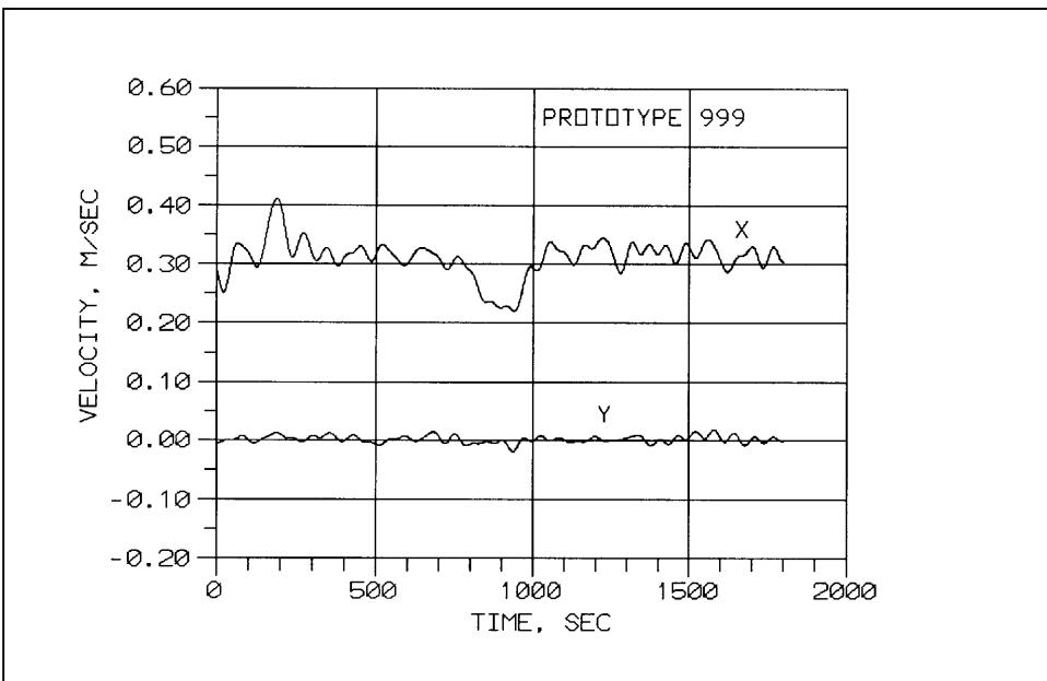
Figure 24. Velocity time history for *Coop Ambassador*, Probe number 999, prototype data
