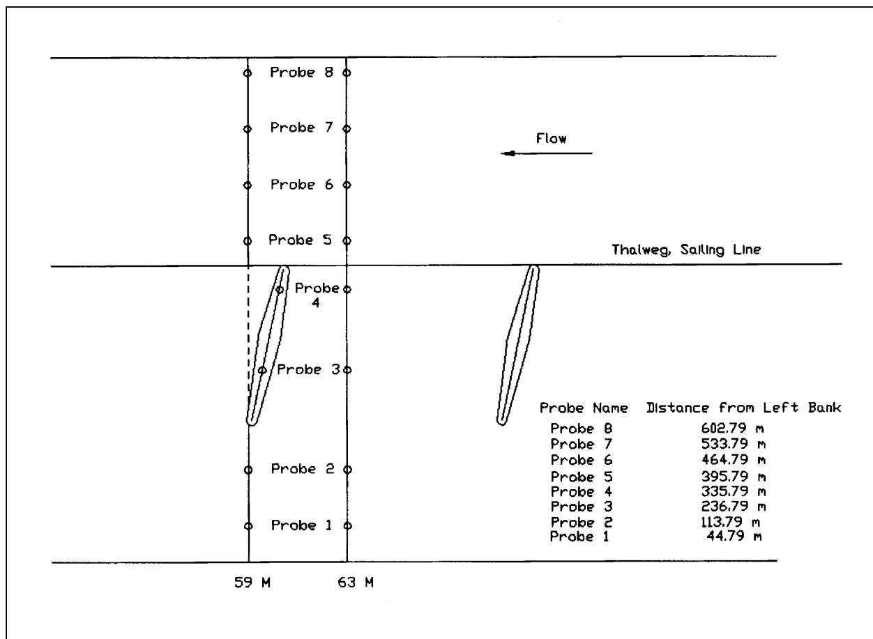
Figure 91. Plan view, experimental series 6
