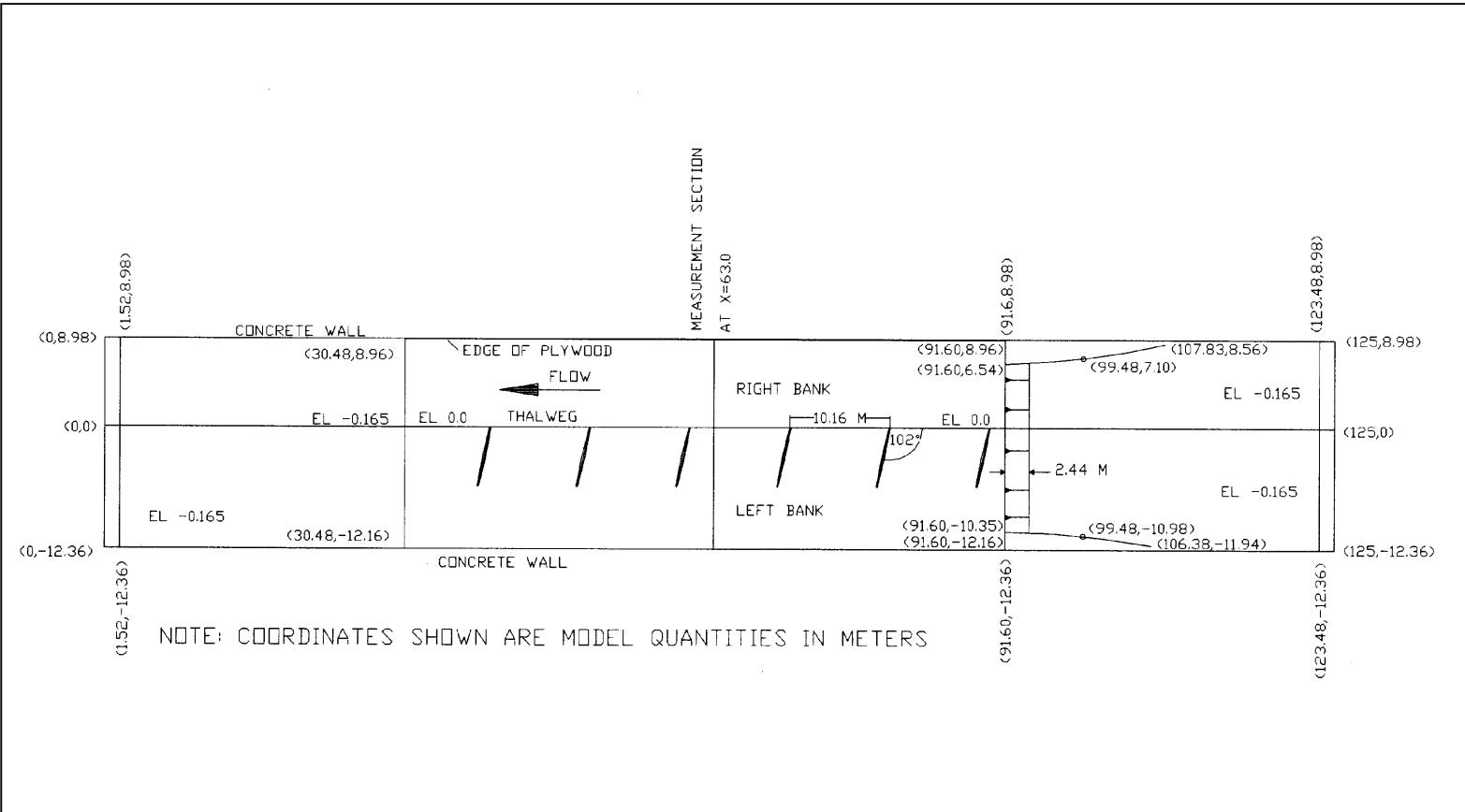
Figure 6. Plan view of 1:30 scale model of Clark's Ferry
