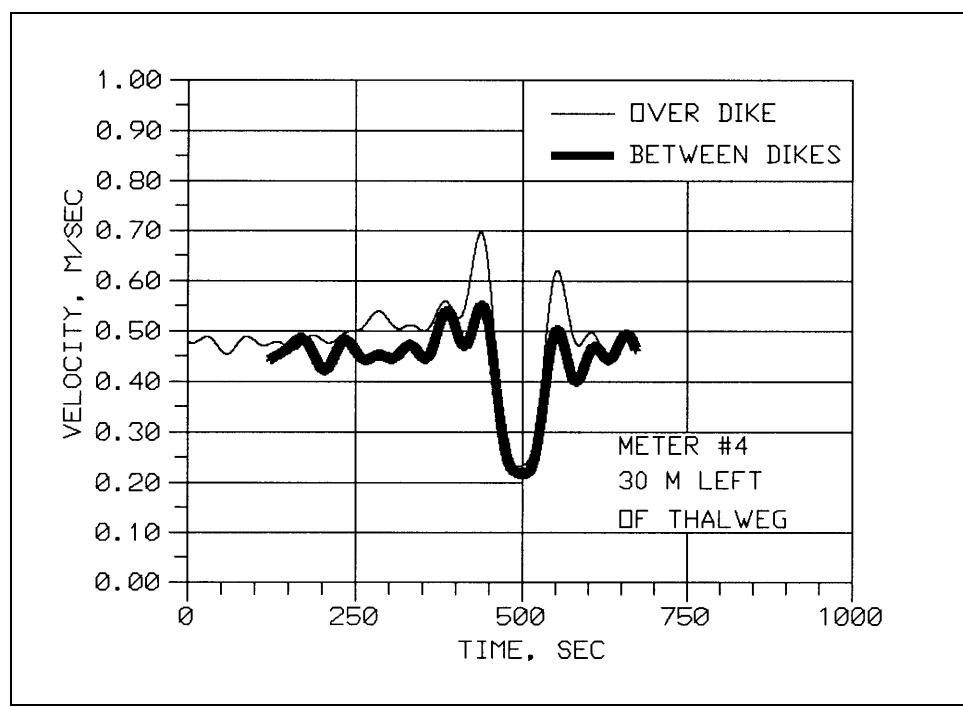
Figure 96. Velocity time history, downbound tow, meter No. 4, tow speed relative to ground = 4.77 m/sec
