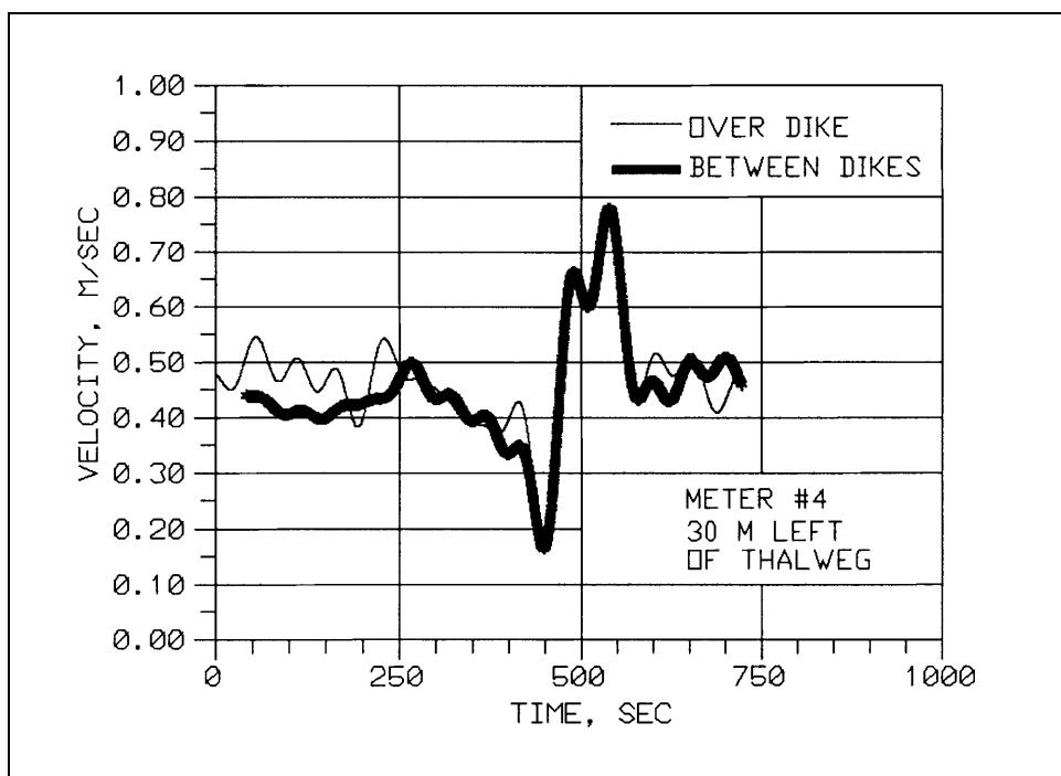
Figure 94. Velocity time history, upbound tow, meter No. 4, tow speed relative to ground = 4.16 m/sec
