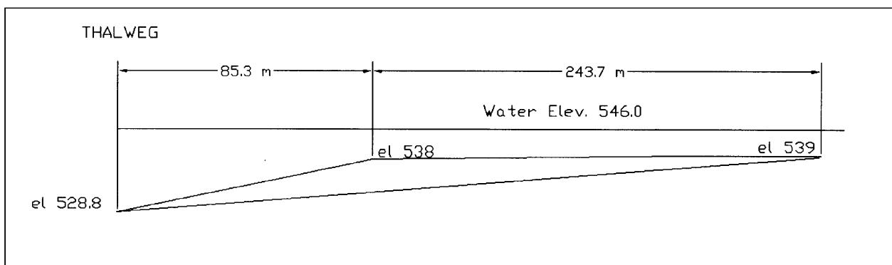
Figure 98. Profile of low dike (looking upstream)
