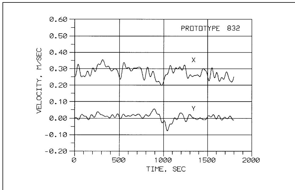
Figure 16. Velocity time history for *Coop Ambassador*, Probe number 832, prototype data
