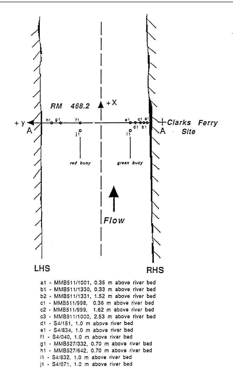
Figure 4. Plan view of the Clark's Ferry site for trip 1 (locations of the current meters are shown)
