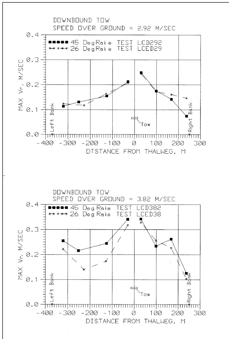
Figure 75. Return velocity, rake angle effects, downbound tow
