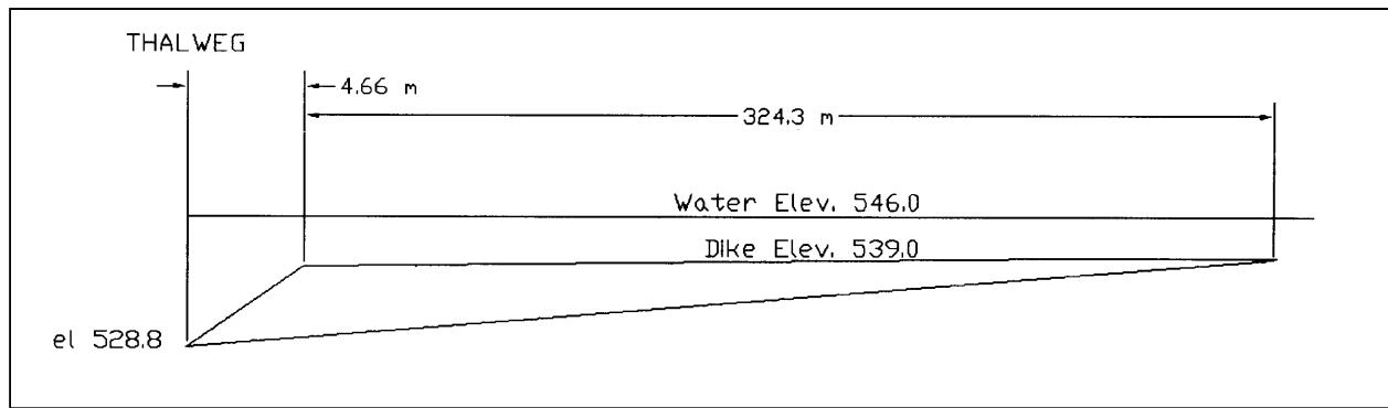
Figure 99. Profile of high (generic) dike (looking upstream)
