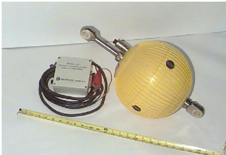
Figure A2. InterOcean S-4 current meter
