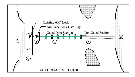
Figure 2. Alternative New Lock Locations at a Typical Existing Lock and Dam Site.
