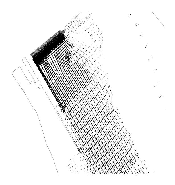
Figure 4 - Example Velocity Vector Plot Showing Flow Through a Location 4 Ported Guardwall at Lock and Dam 22.
