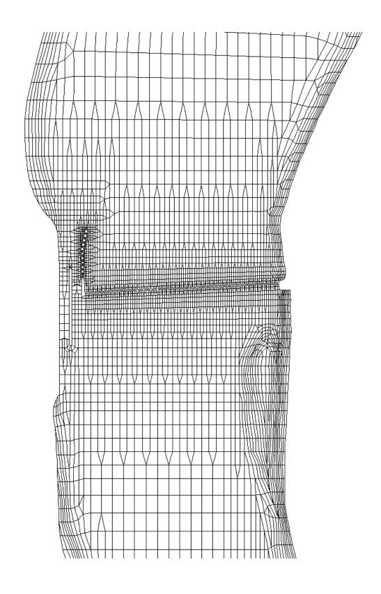
Figure 2 - Portions of the Head and Tailwater Finite Element Meshes for Lock and Dam 20, Base Conditions.
