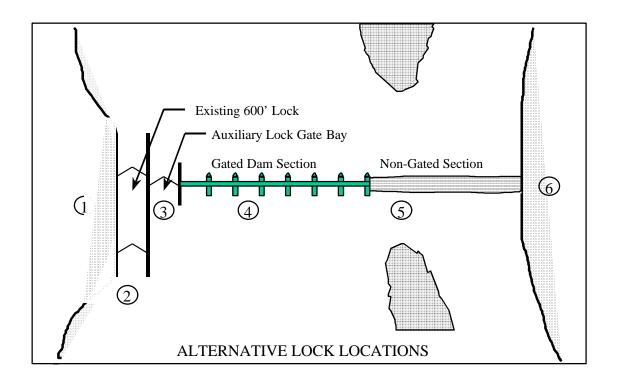
Figure 1 - Alternative New Lock Locations at a Typical Existing Lock and Dam Site.
