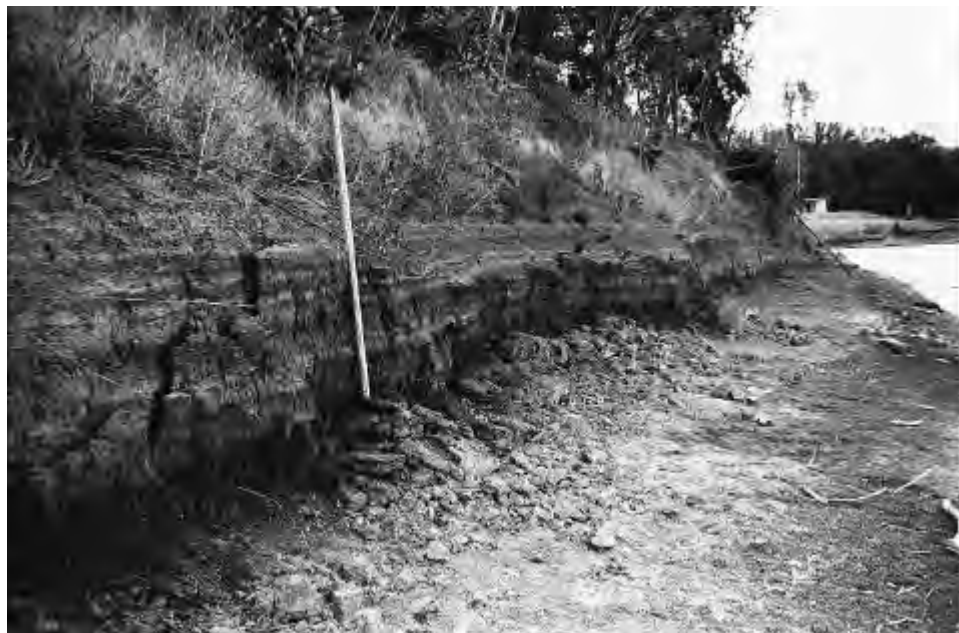
Photo 7-8 Thick historical alluvium overlying the native soil observed at Observation Site, RM 194.0 (the bottom of stadia rod indicates the native soil surface)
