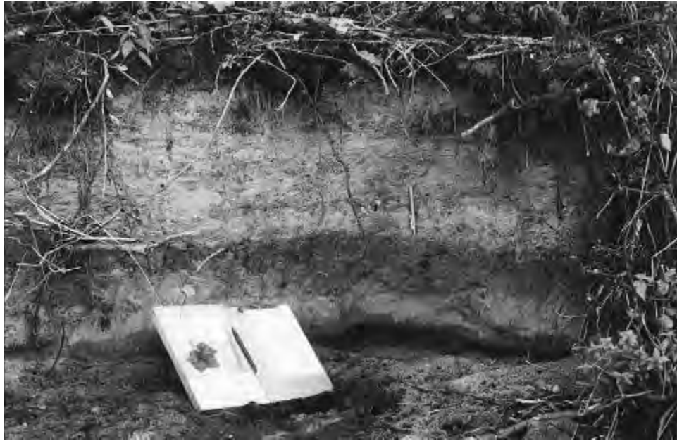
Photo 7-6 Buried native soil below historical alluvium observed at Site 4, RM 751.1 (the lighter colored upper unit is the historical deposit)
