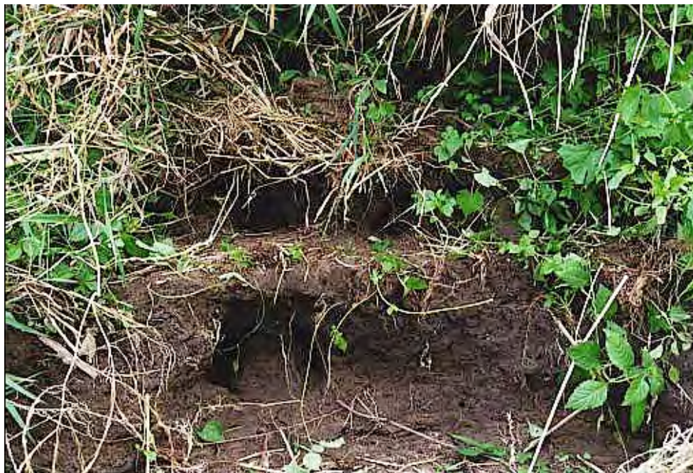
Photo 7-36 Piping feature of Site 14 midpoint
