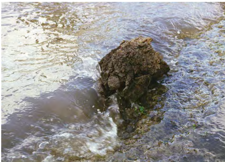
Photo 7-97 A block of failed bank soil placed in water (t = 2 min.) -- Observation Site at RM 195.1 LDB
