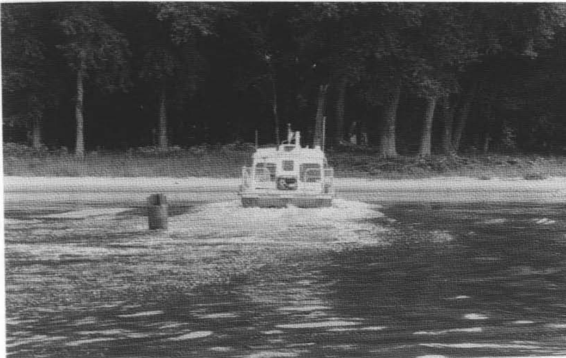
Figure 3-10. River cross section measurement by A ISWS boat equipped with the GPS and Sonnar
