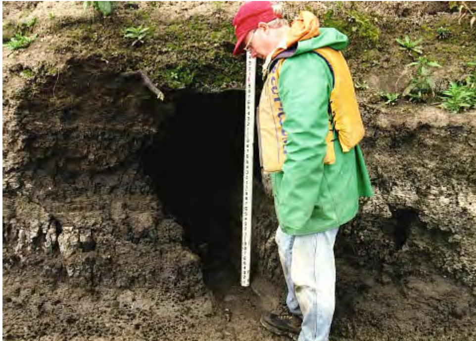
Photo 7-74 Further close-up of piping features - Observation Site at RM 322.9 RDB
