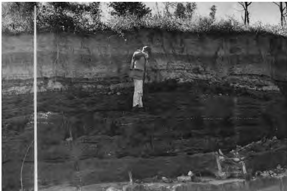
Photo 7-10 Bank face showing a profile composed entirely of recent historical alluvium at Site 39, RM 112.4
