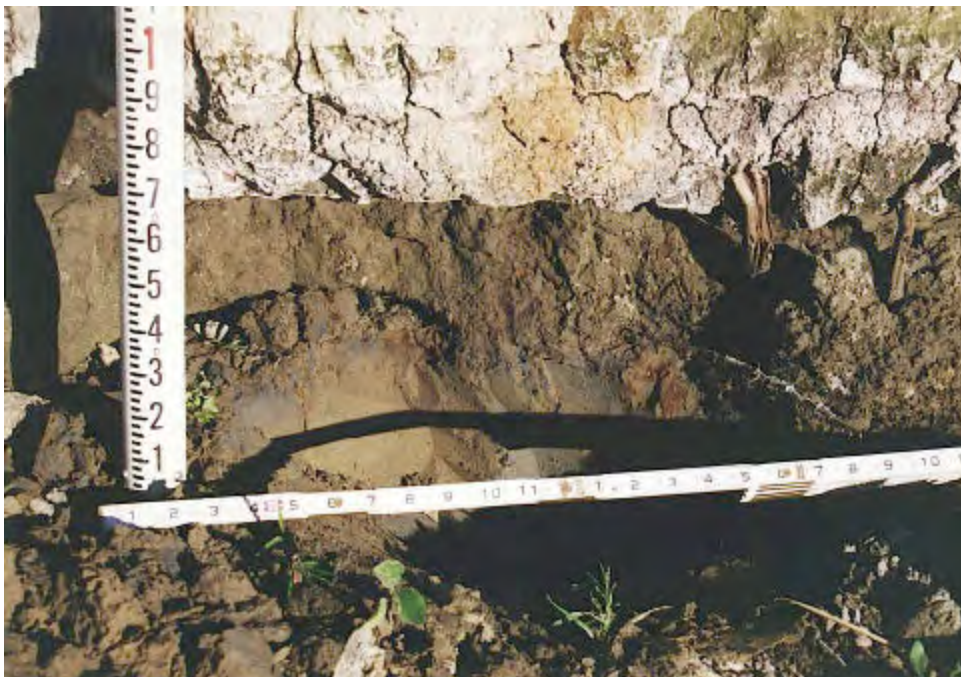
Photo 7-106 Sand lens found at terrace of Observation Site at RM 168.5 LDB
