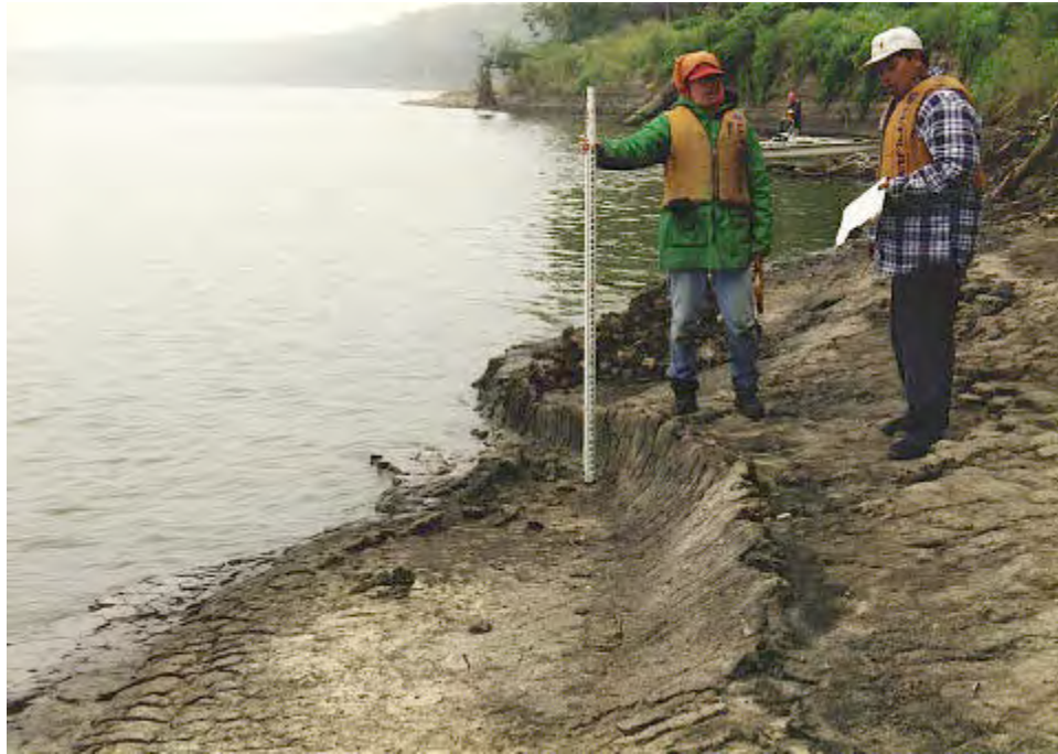
Photo 7-70 Bench smeared by a barge - Observation Site at RM 322.9 RDB
