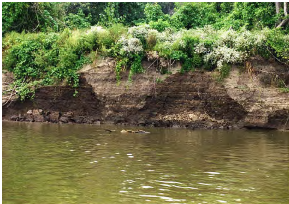
Photo 7-75 Vertical bank failure - Observation Site at RM 322.9 RDB
