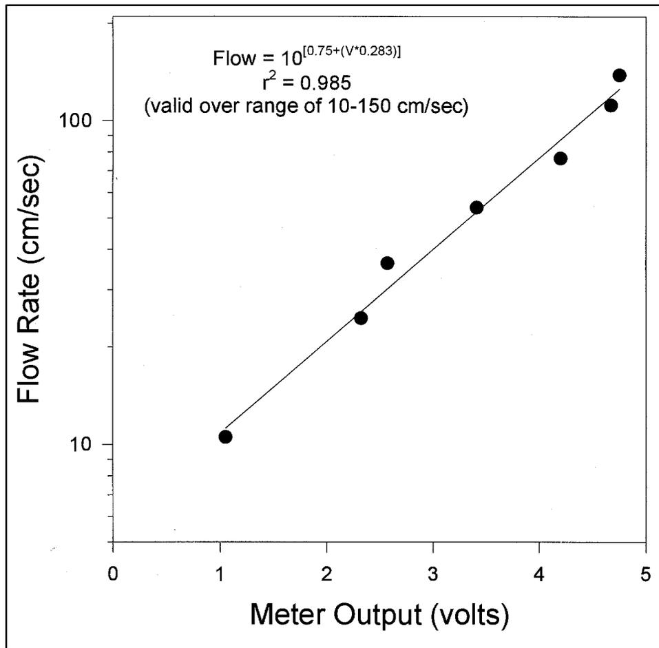
Figure 2. Calibration of flow velocity sensor over range of 10-150 cm sec<sup>-1</sup>
