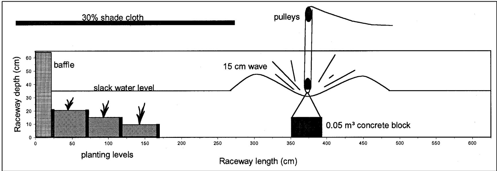
Figure 1. Design of experimental raceway
