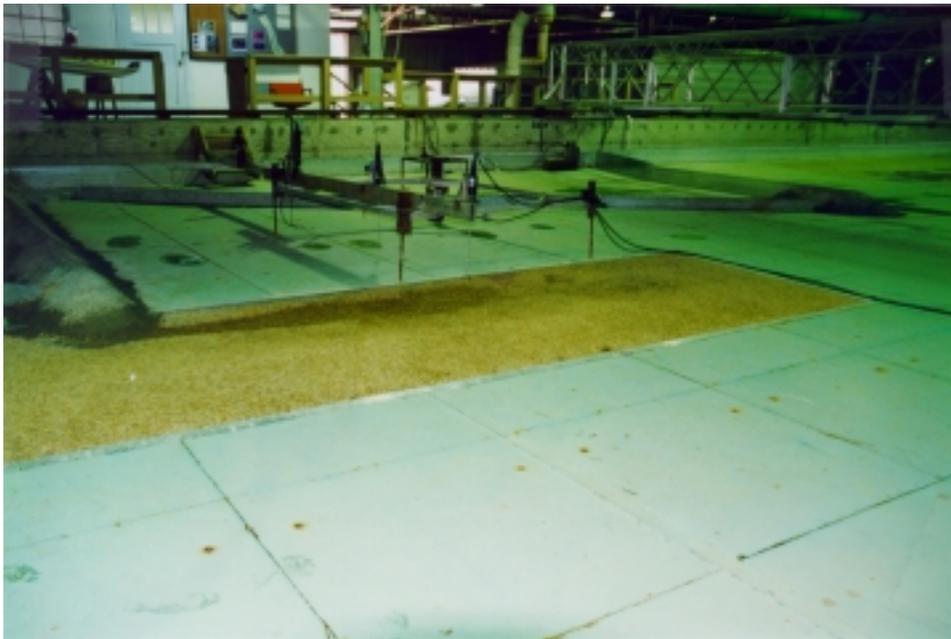
b. Side view, experimental dike at left, downstream dike at right, scour hole in gravel
