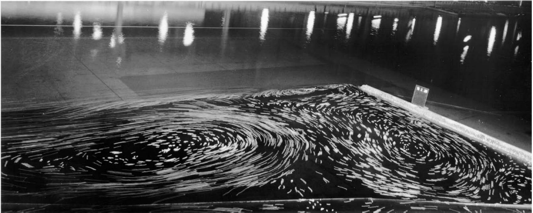
Photo 3. L-head dike, 137 m long by 3.5 m high, without tow
