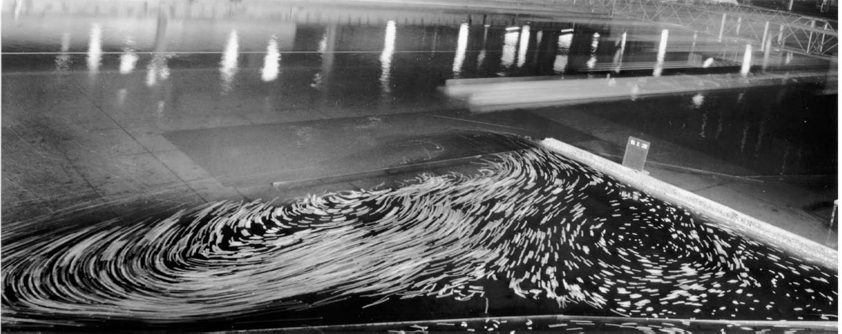
Photo 4. L-head dike, 137 m long by 3.5 m high, with tow
