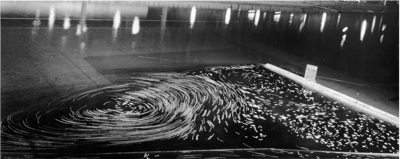
Photo 9. L-head dike, 69 m long by 1.7 m high, without tow
