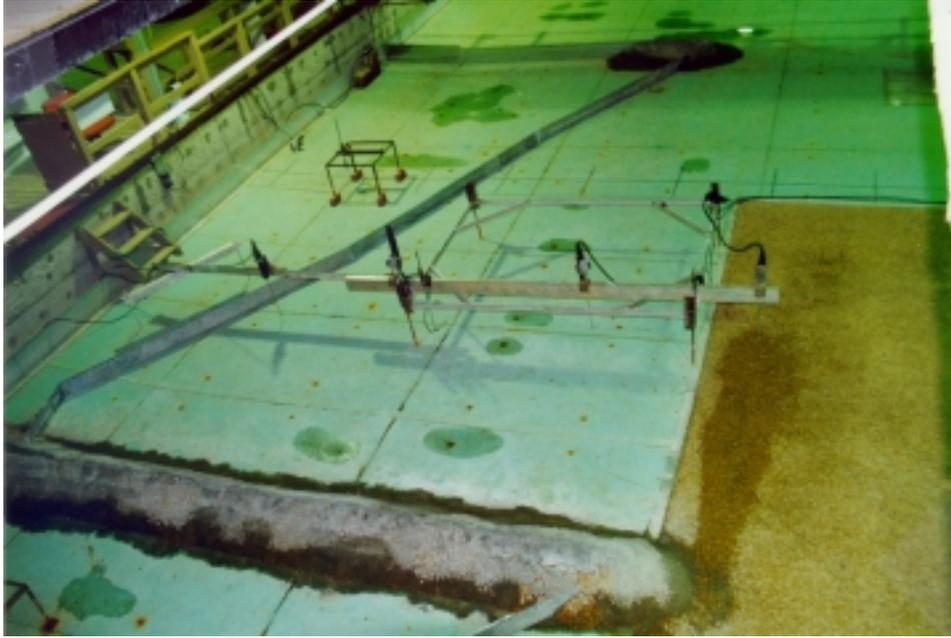
a. Overhead view looking downstream, experimental dike at bottom, downstream dike at top
