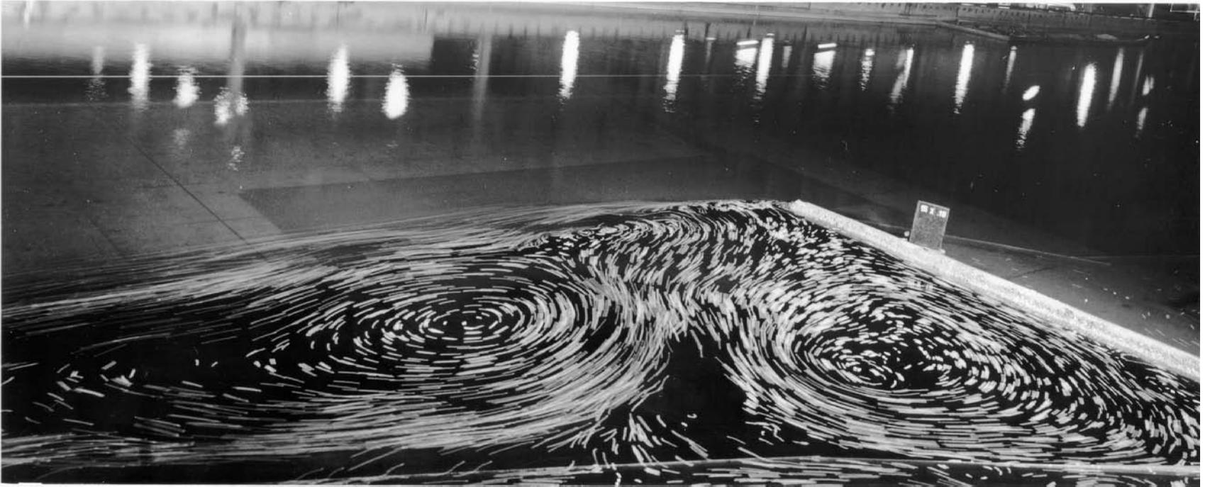
Photo 5. L-head dike, 137 m long by 1.7 m high, without tow
