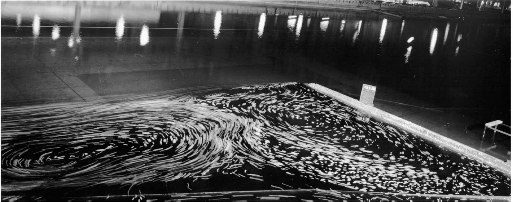
Photo 7. L-head dike, 69 m long by 3.5 m high, without tow
