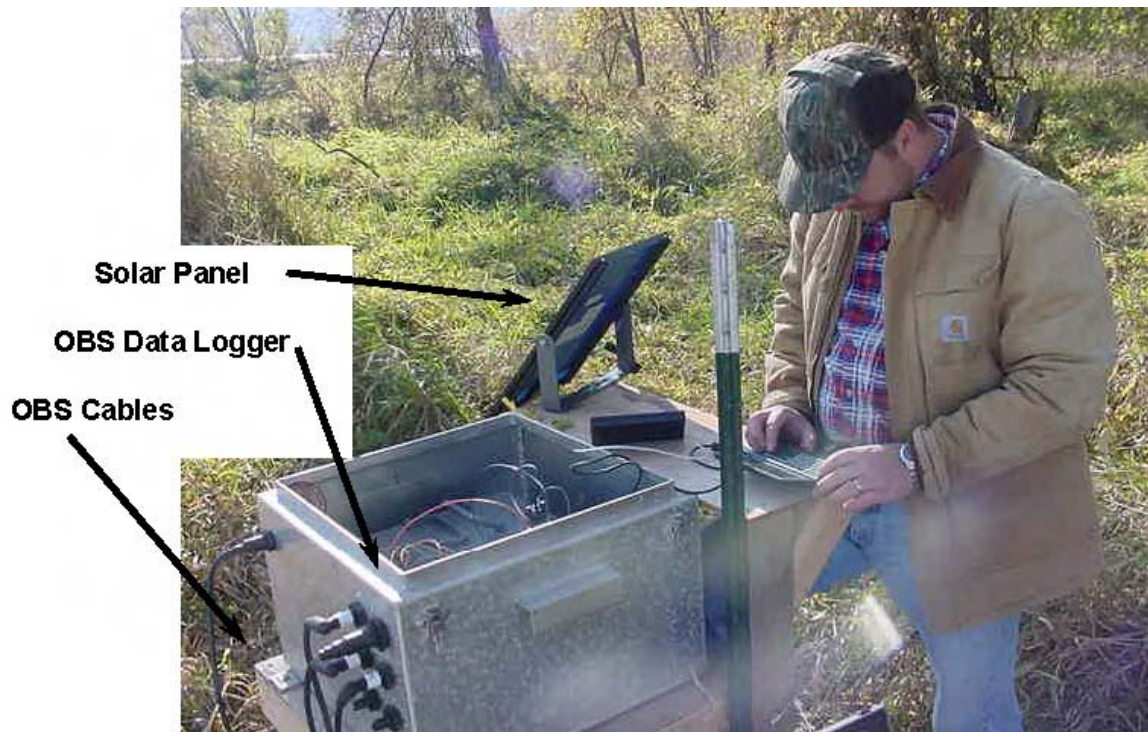
Photo A3. Setting up the data logger for the OBS sensors
