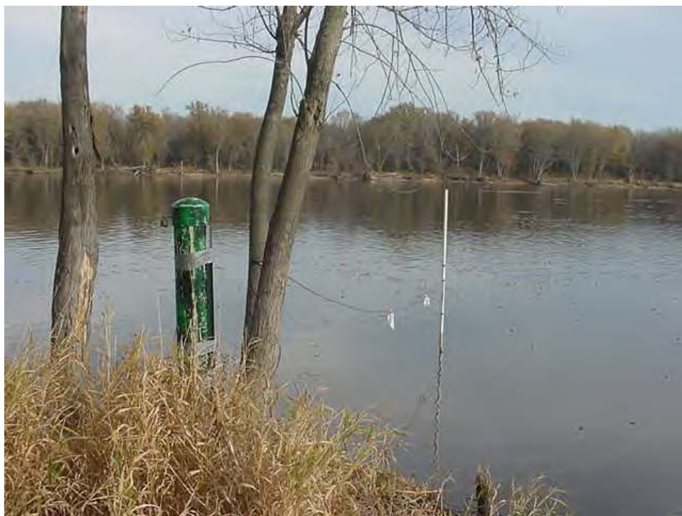
Photo A9. Water level recorder and sensor deployment at Pool 13
