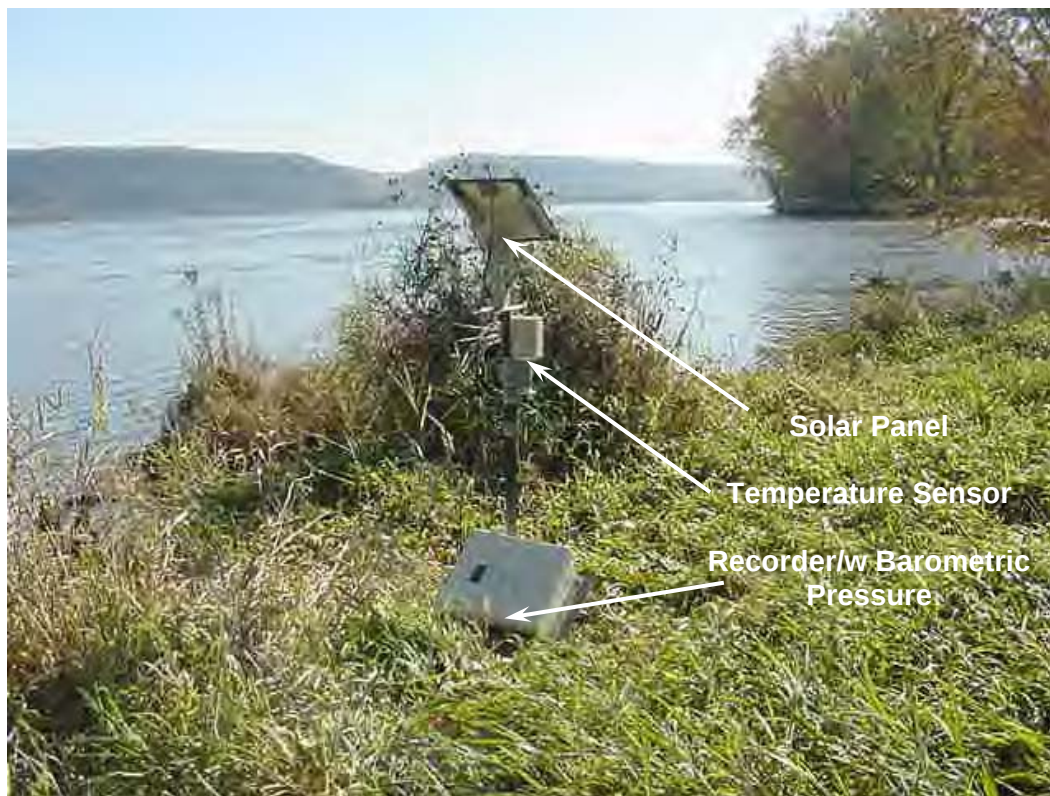
Photo A4. Meteorological recording station for Site 1 and 2, Pool 10
