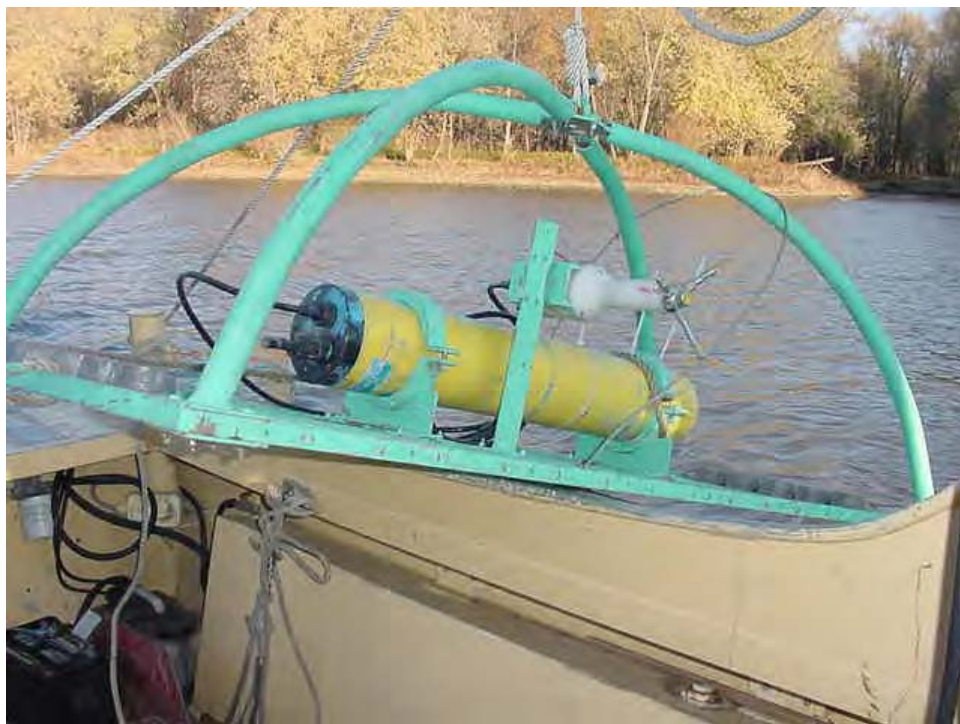
Photo A12. Deployment mount with ADV ready for deployment at Pool 13 Site 2
