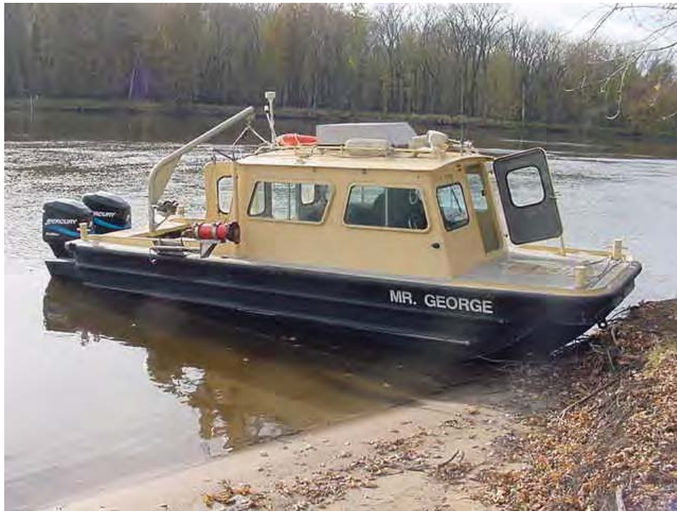
Photo A11. Data collection boat and ADCP sensor for discharge measurements
