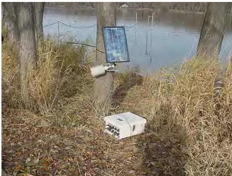
Photo A10. Meteorological recording station for Site 1 and 2, Pool 13
