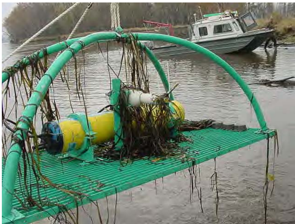
Photo A5. Deployment mount with ADV being retrieved for cleaning
