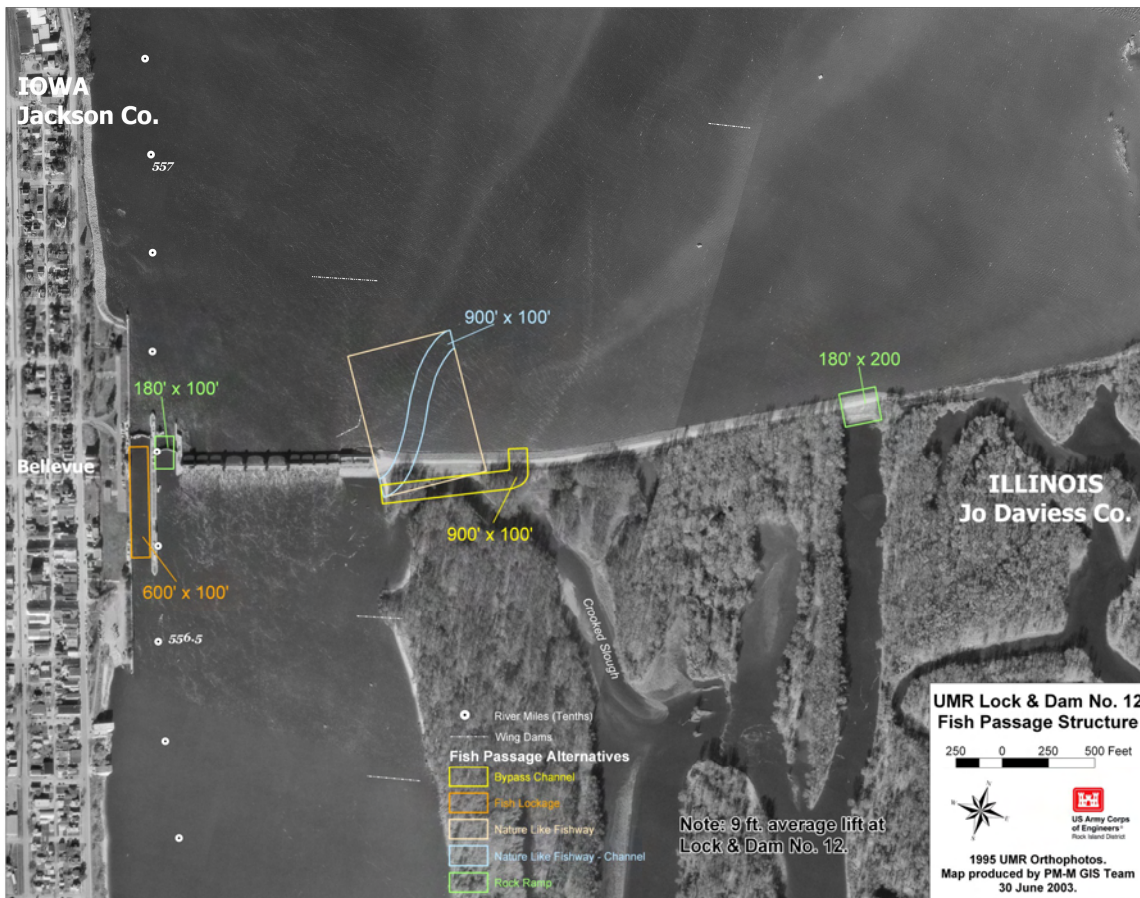
Figure D13. Potential fish passage improvements at Lock and Dam 12, Upper Mississippi River
