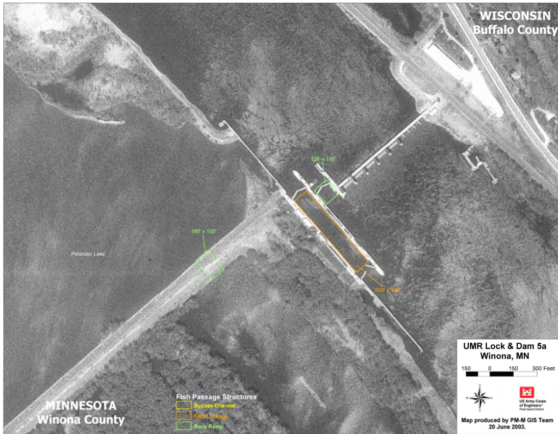
Figure D6. Potential fish passage improvements at Lock and Dam 5A, Upper Mississippi River
