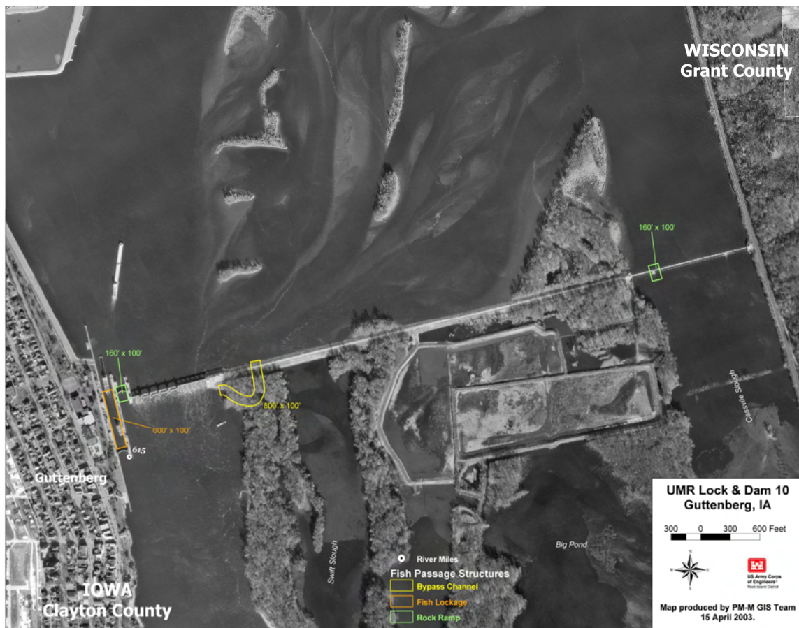
Figure D11. Potential fish passage improvements at Lock and Dam 10, Upper Mississippi River
