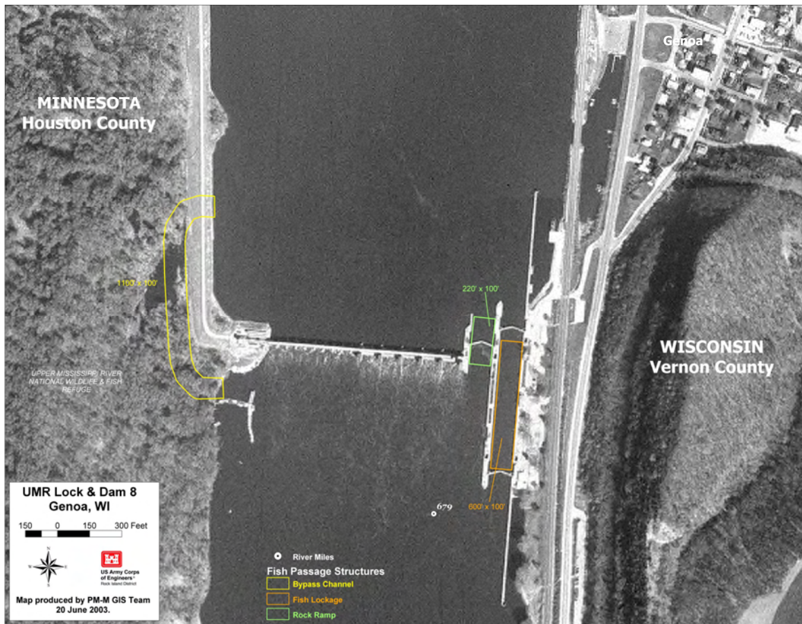
Figure D9. Potential fish passage improvements at Lock and Dam 8, Upper Mississippi River
