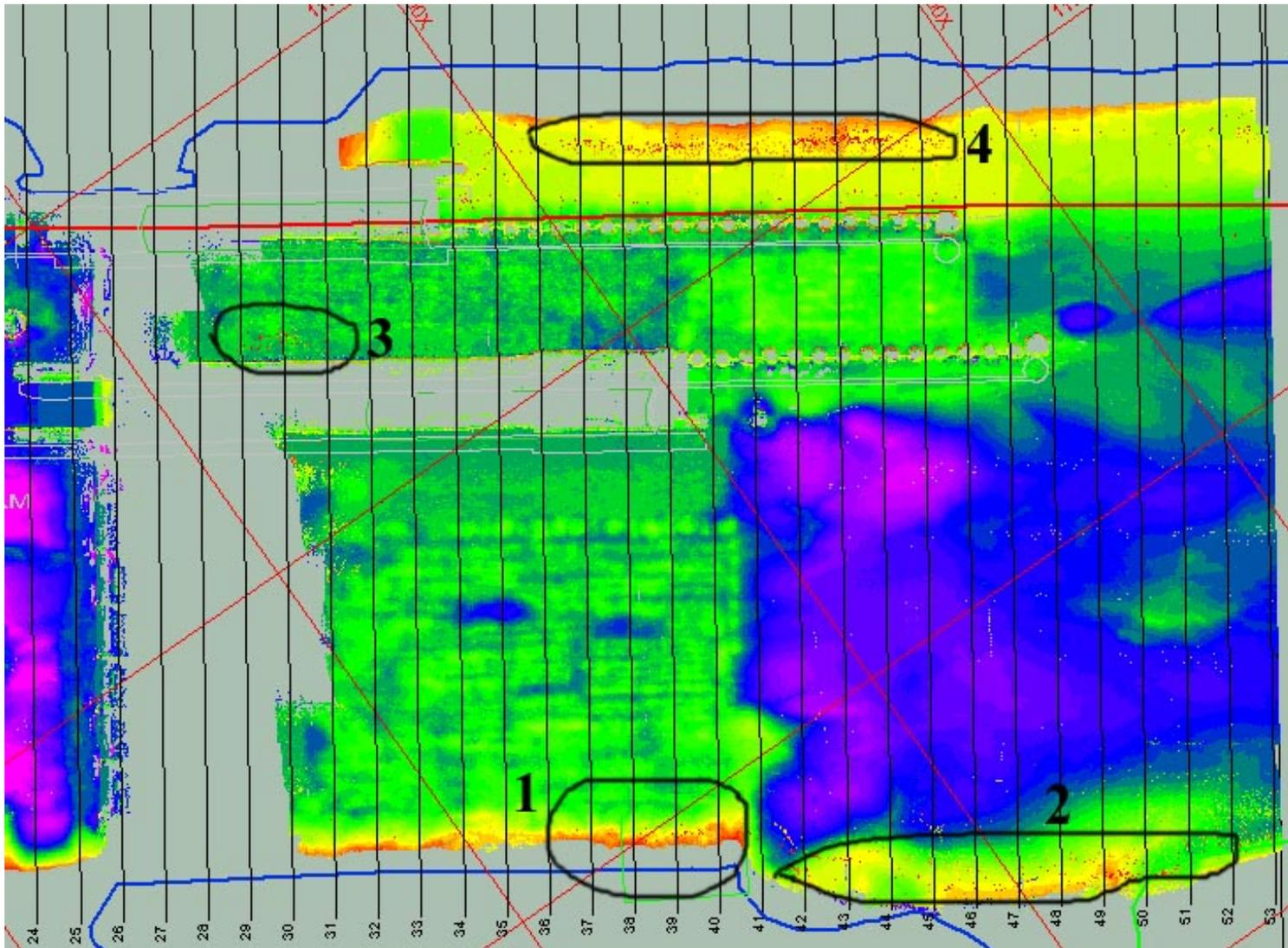
**Figure 1.** Bathymetric Survey Map of the Tailwater Area of Melvin Price Locks and Dam – May 25, 2005
